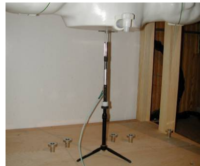
Figure 10-2 System Verification Setup Photo
