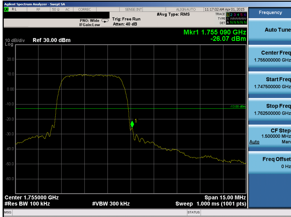
Plot 6-63. Band Edge Plot (AWS WCDMA Mode – Ch. 1862)
