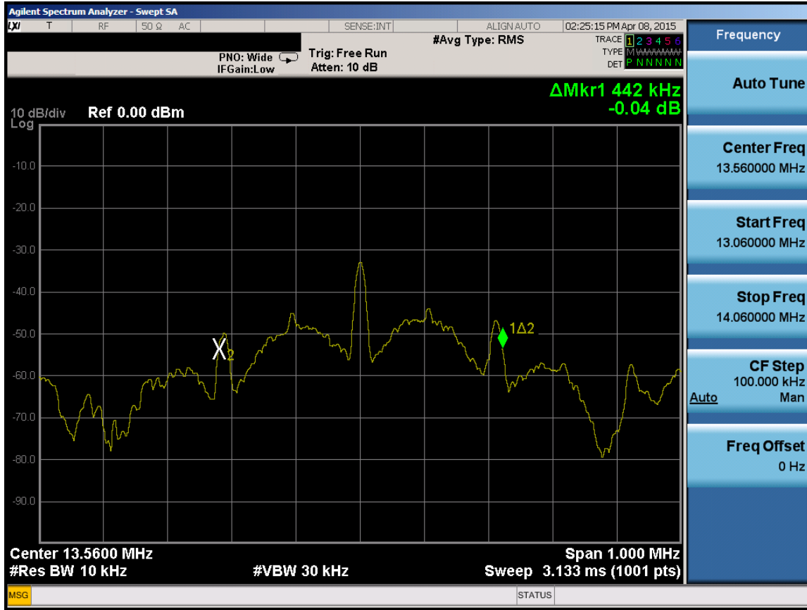
Figure 7-3. 20dB Bandwidth Plot with WCP
