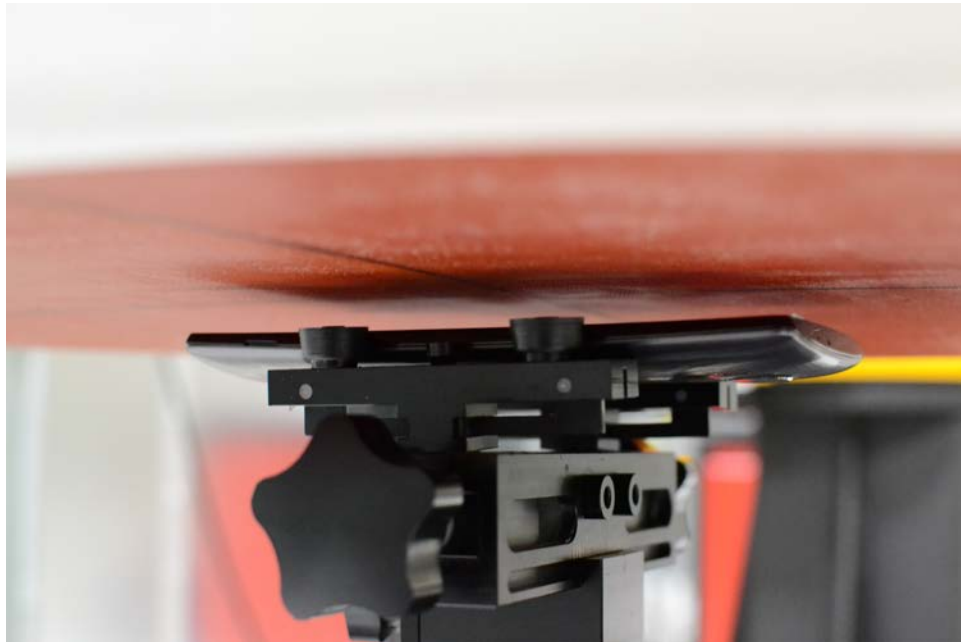
SAR Test Setup Photo 18: Front Side, Standard Cover at 10 mm
