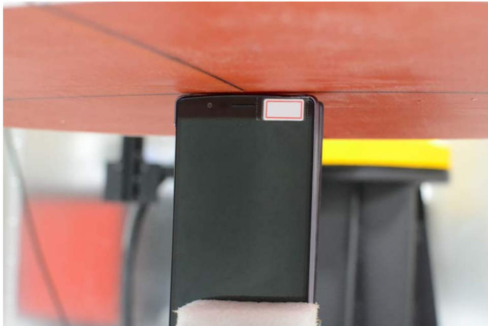
SAR Test Setup Photo 24: Top Edge, Quick Cover (Open) at 0 mm
