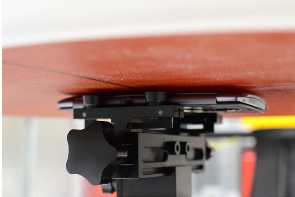
SAR Test Setup Photo 17: Back Side, Quick Cover (Closed) at 0 mm
