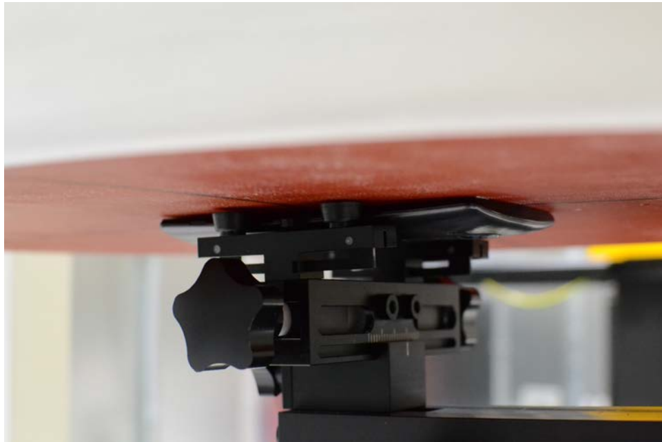
SAR Test Setup Photo 20: Front Side, Standard Cover at 0 mm
