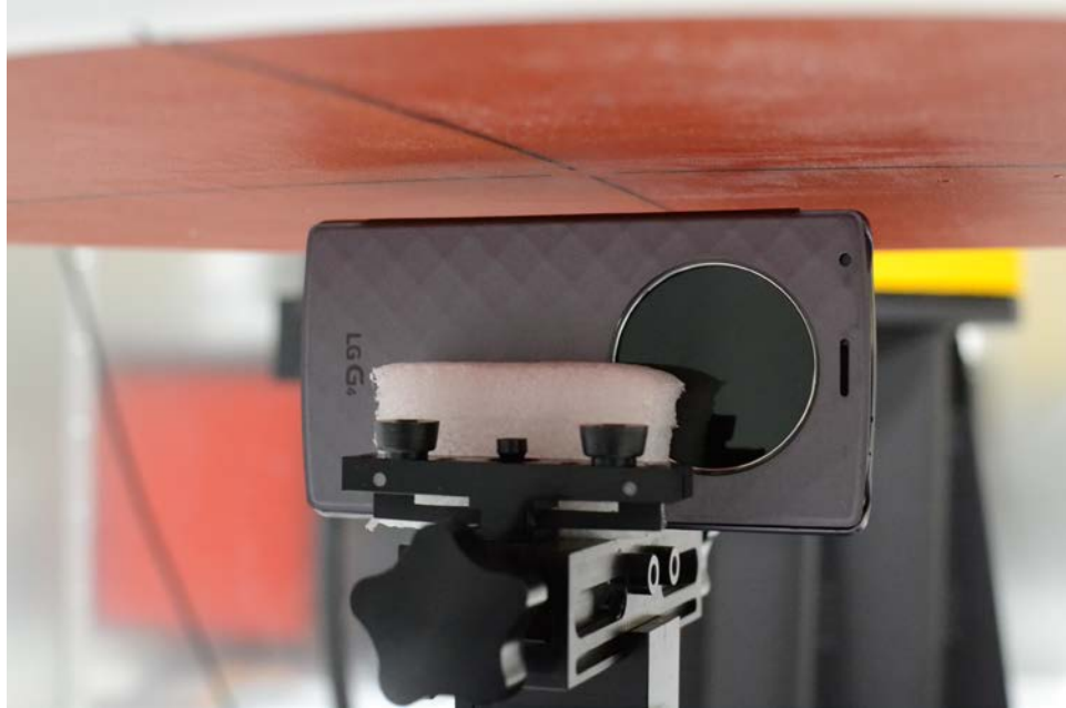
SAR Test Setup Photo 31: Left Edge, Quick Cover (Closed) at 10 mm
