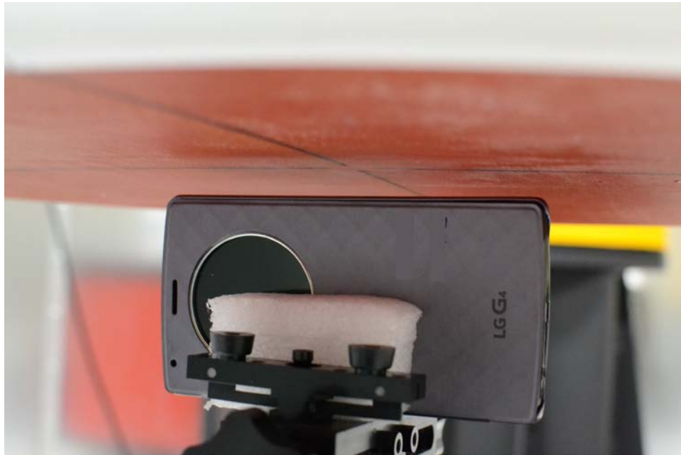
SAR Test Setup Photo 28: Right Edge, Quick Cover (Closed) at 10 mm
