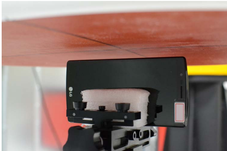
SAR Test Setup Photo 26: Left Edge, Standard Cover at 10 mm
