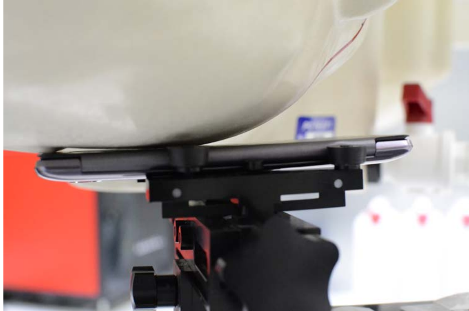
SAR Test Setup Photo 3: Right Cheek, Quick Cover (Closed)
