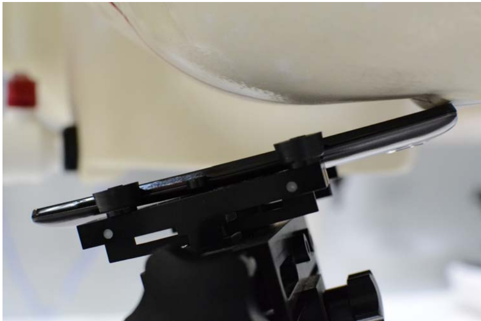
SAR Test Setup Photo 10: Left Tilt, Standard Cover
