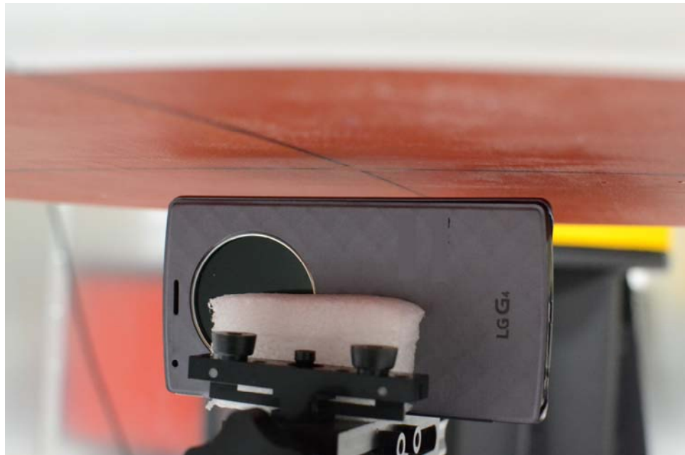
SAR Test Setup Photo 24: Right Edge, Quick Cover (Closed) at 10 mm
