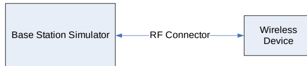
Figure 9-1 Power Measurement Setup
