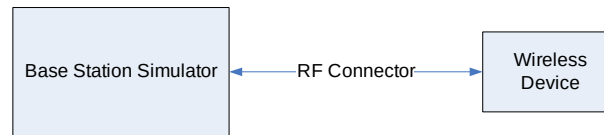
Figure 9-2 Power Measurement Setup
