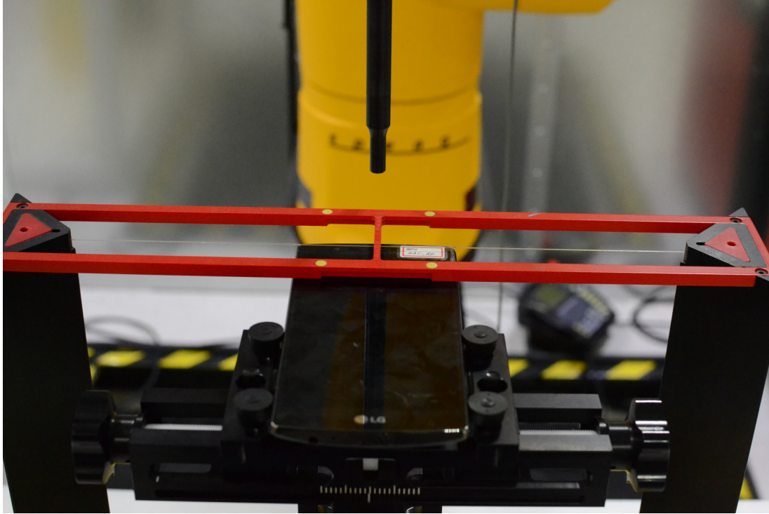
Figure 17-1 Ear Reference Point HAC Phantom Alignment, Standard Cover
