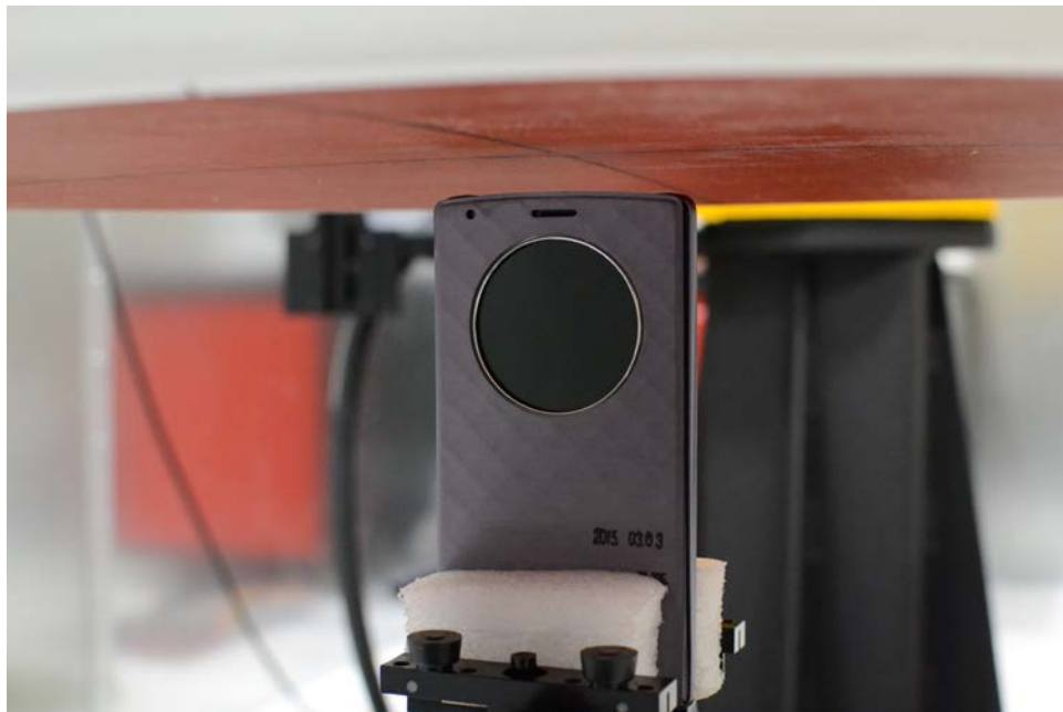
SAR Test Setup Photo 20: Top Edge, Quick Cover (Closed) at 10 mm
