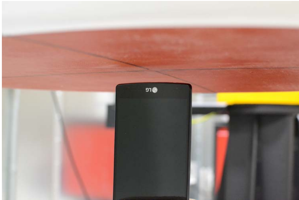
SAR Test Setup Photo 24: Bottom Edge, Standard Cover at 10 mm
