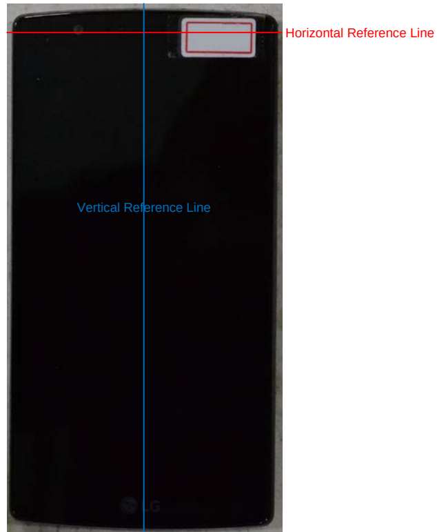
SAR Test Setup Photo 28: Horizontal and Vertical Reference Lines
