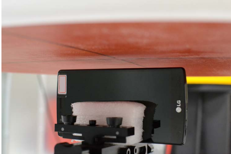
SAR Test Setup Photo 25: Right Edge, Standard Cover at 10 mm
