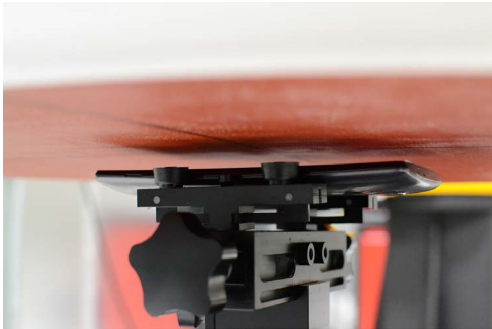
SAR Test Setup Photo 16: Front Side, Standard Cover at 10 mm
