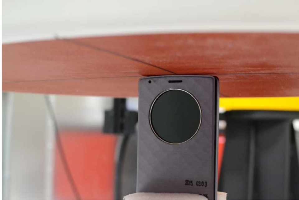
SAR Test Setup Photo 23: Top Edge, Quick Cover (Closed) at 0 mm
