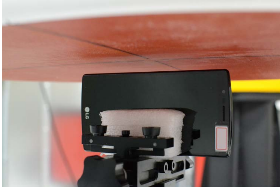
SAR Test Setup Photo 27: Left Edge, Standard Cover at 10 mm
