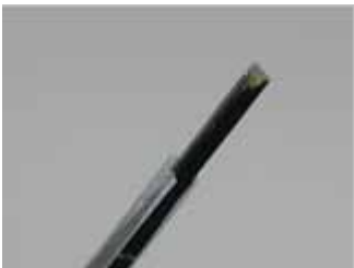
Figure 6. EX3DV4 E-field Probe
