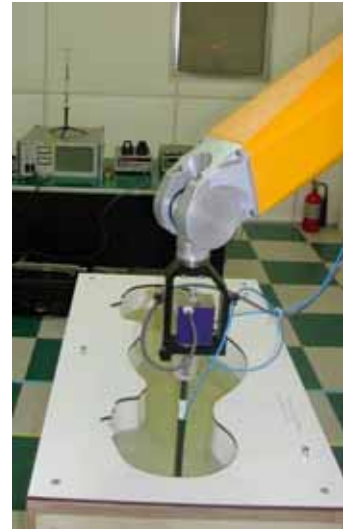
Figure 3. Photograph of the probe and the Phantom
