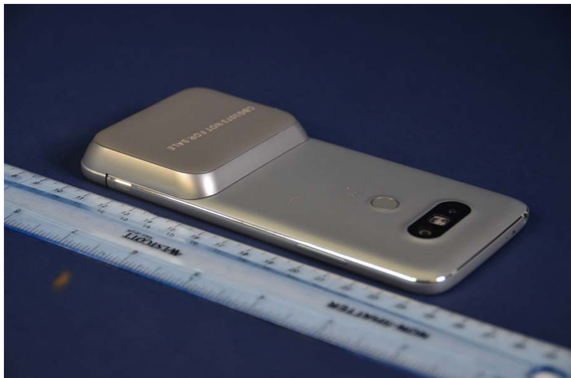
Camera Module Installed
