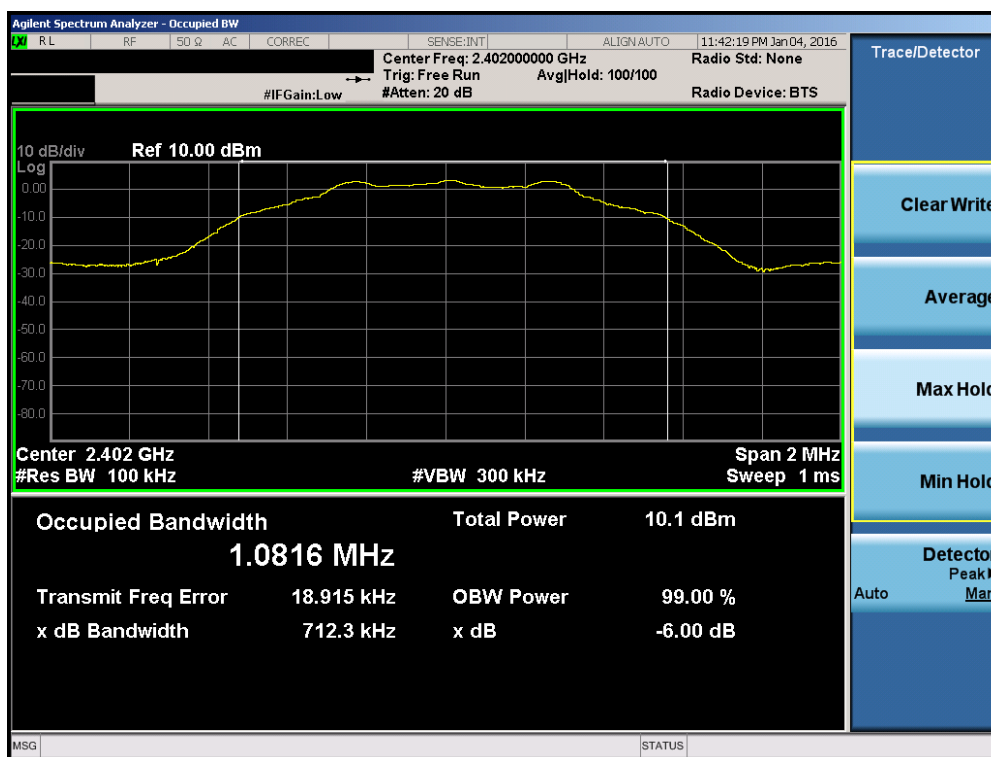
Plot 7-1. 6dB Bandwidth Plot (Bluetooth (LE) – Ch. 0)
