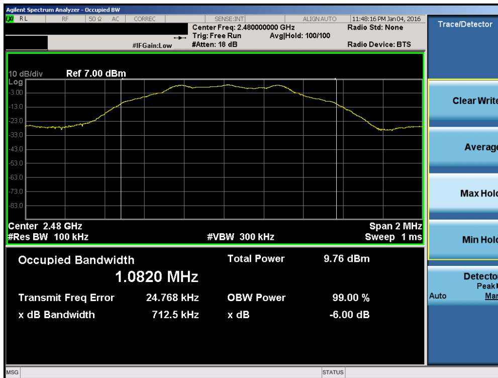
Plot 7-3. 6dB Bandwidth Plot (Bluetooth (LE) – Ch. 39)
