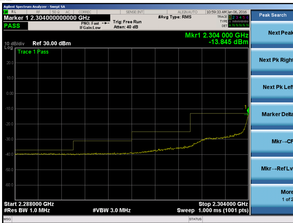
Plot 7-186. Lower Extended Band Edge Plot (Band 30 – 5.0MHz QPSK – RB Size 25)
