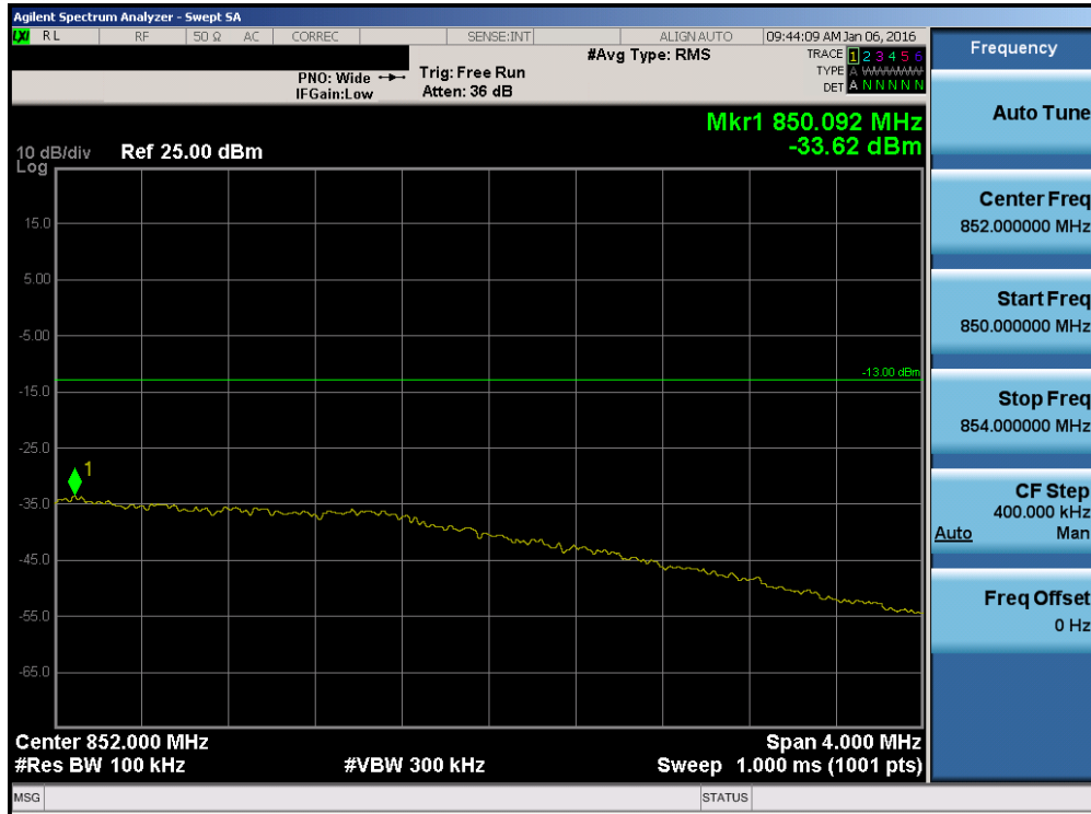
Plot 7-130. Upper Extended Band Edge Plot (Band 5 – Band 5 – 3.0MHz QPSK – RB Size 15)
