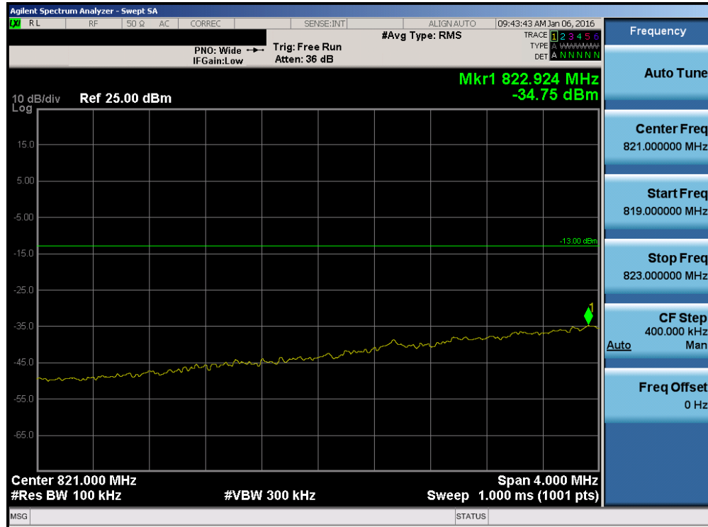
Plot 7-128. Lower Extended Band Edge Plot (Band 5 – 3.0MHz QPSK – RB Size 15)
