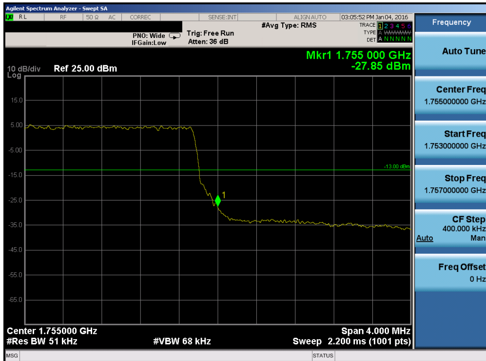
Plot 7-147. Upper Band Edge Plot (Band 4 – 5.0MHz QPSK – RB Size 25)
