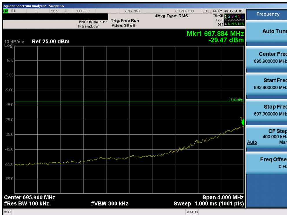
Plot 7-108. Lower Extended Band Edge Plot (Band 12 – 1.4MHz QPSK – RB Size 6)
