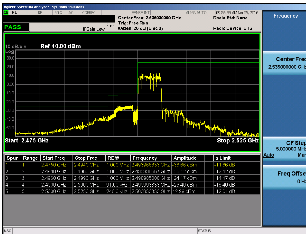
Plot 7-193. Lower ACP Plot (Band 7 – 5.0MHz QPSK – RB Size 25)
