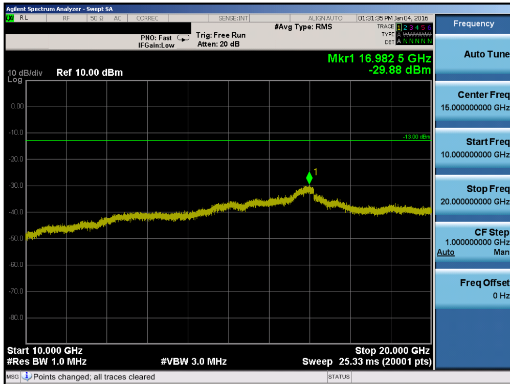
Plot 7-49. Conducted Spurious Plot (PCS WCDMA Mode – Ch. 9400)
