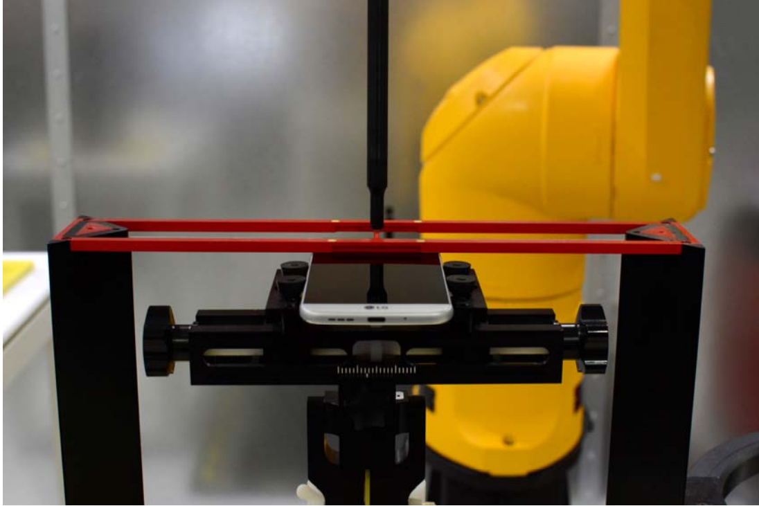
Figure 18-1 Ear Reference Point HAC Phantom Alignment
