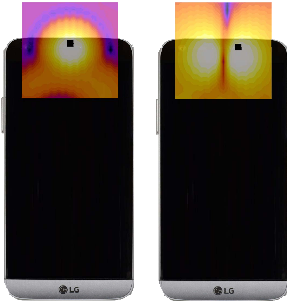
Figure 14-5 T-Coil Scan Overlay Magnetic Field Distributions
