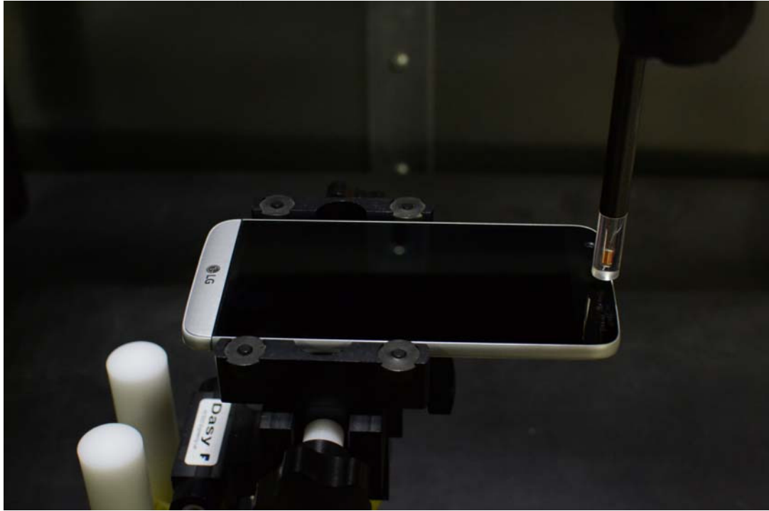
Figure 14-1 Test Setup for Wireless Device
