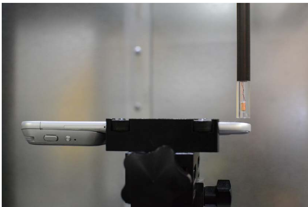
Figure 14-4 Test Setup for Wireless Device – Camera Module Accessory
