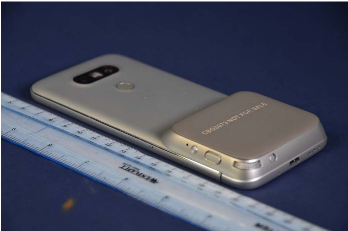
Camera Module Installed
