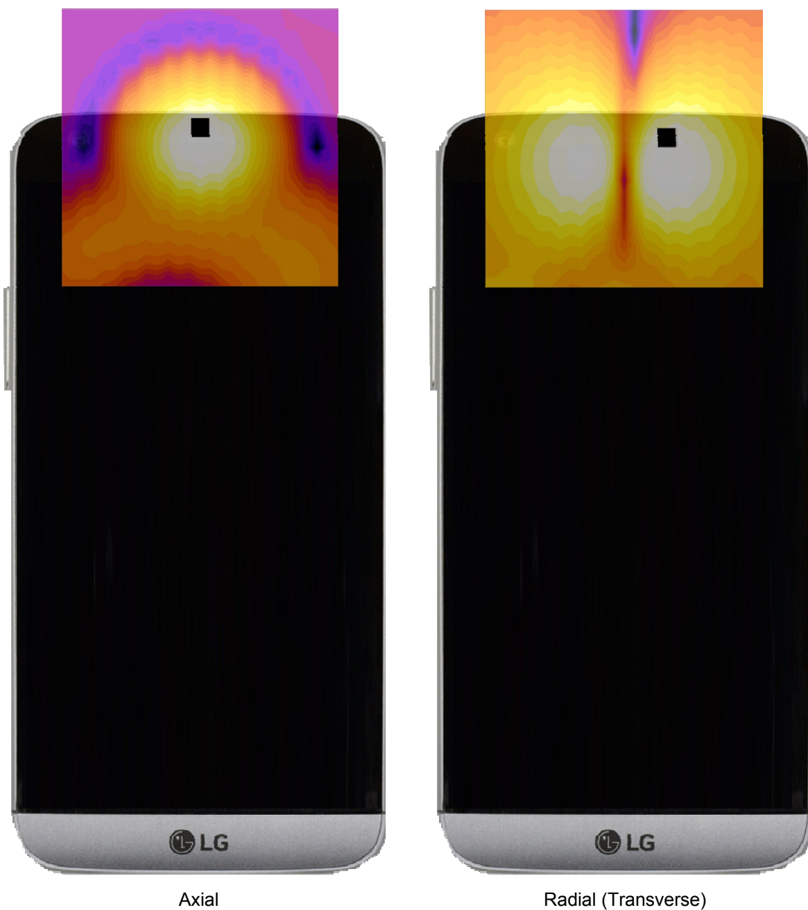
Figure 14-5 T-Coil Scan Overlay Magnetic Field Distributions
