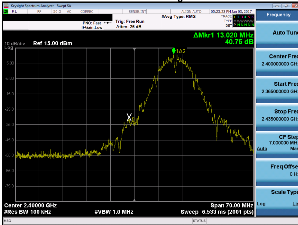
Plot 7-43. Band Edge Plot (802.11b – Ch. 1)
