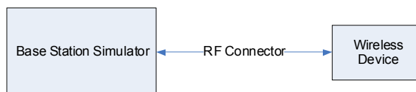
Figure 9-1 Power Measurement Setup
