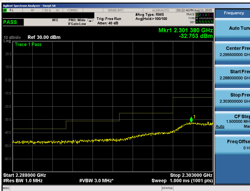
Plot 6-158. Lower Extended Band Edge Plot (Band 30 – 5.0MHz QPSK – RB Size 25)
