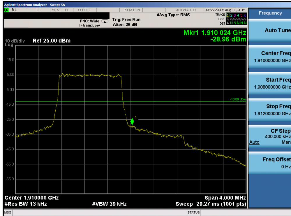
Plot 6-135. Upper Band Edge Plot (Band 2 – 1.4MHz QPSK – RB Size 6)
