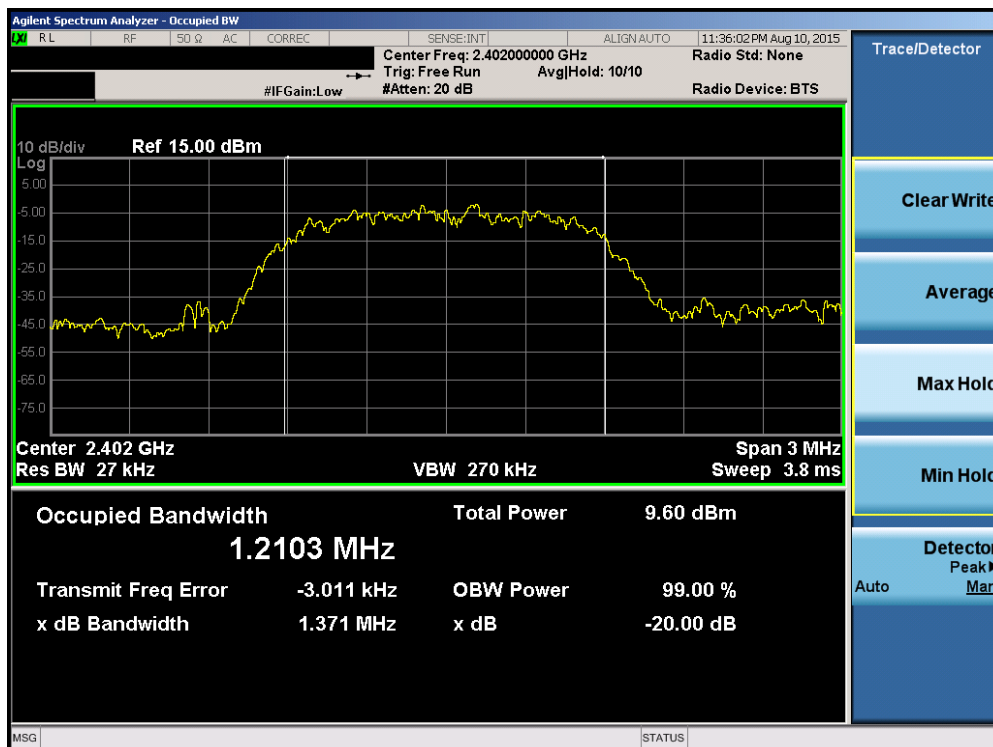
Plot 6-7. 20dB Bandwidth Plot (Bluetooth, 3Mbps – Ch. 0)
