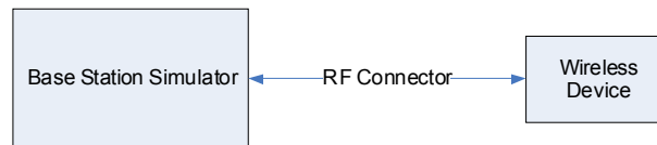
Figure 9-2 Power Measurement Setup
