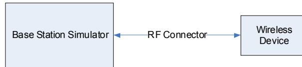
Figure 9-2 Power Measurement Setup
