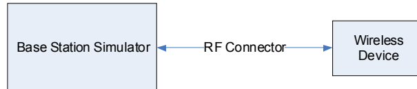
Figure 9-1 Power Measurement Setup
