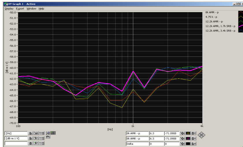
Figure 5-1 UMTS Audio Band Magnetic Noise
