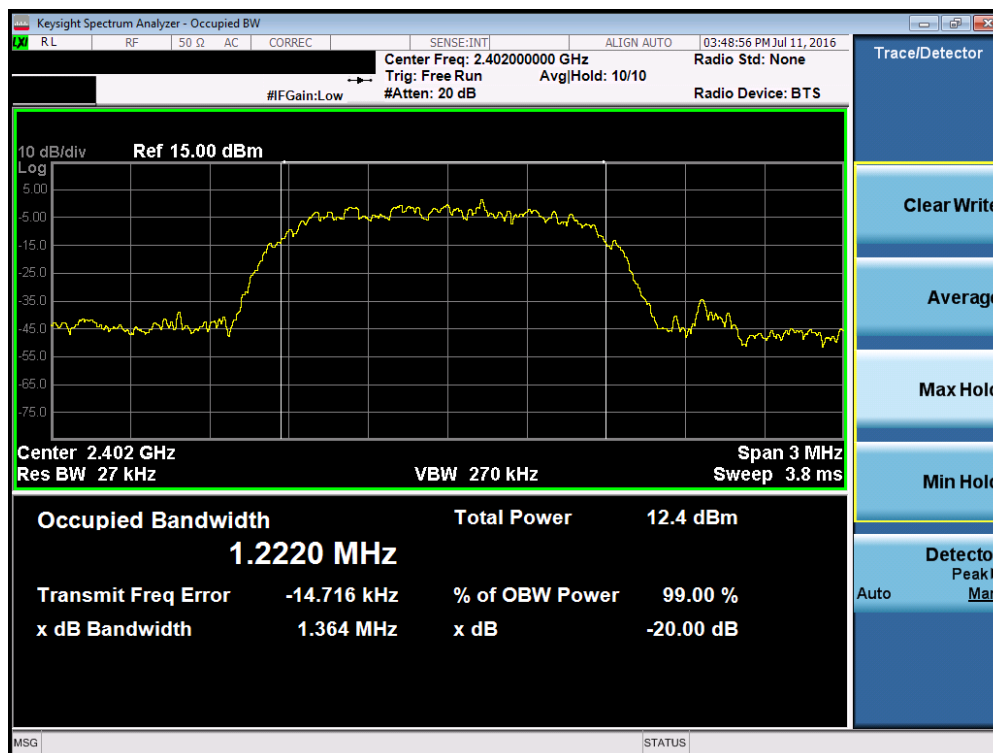
Plot 7-4. 20dB Bandwidth Plot (Bluetooth, 2Mbps – Ch. 0)
