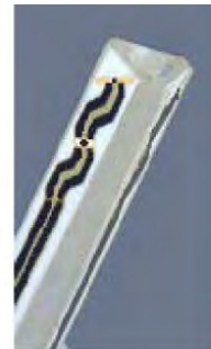
Figure 3.3 Probe Thick-Film Technique
