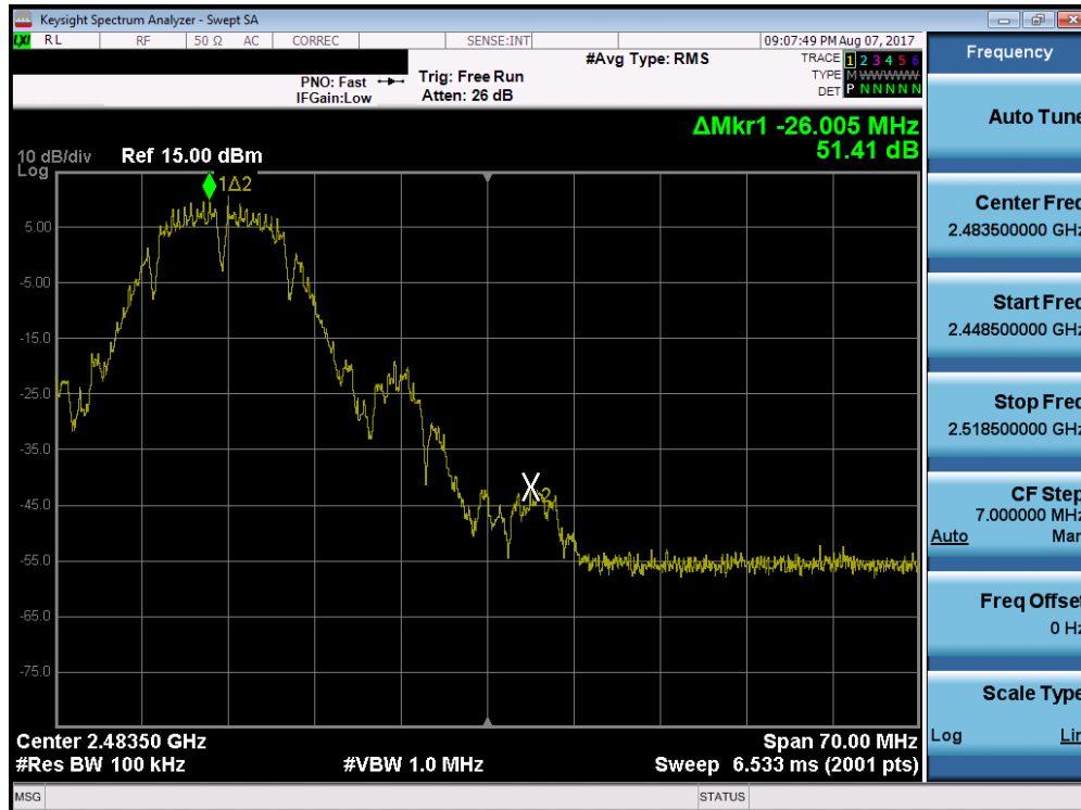
Plot 7-44. Band Edge Plot (802.11b – Ch. 11)
