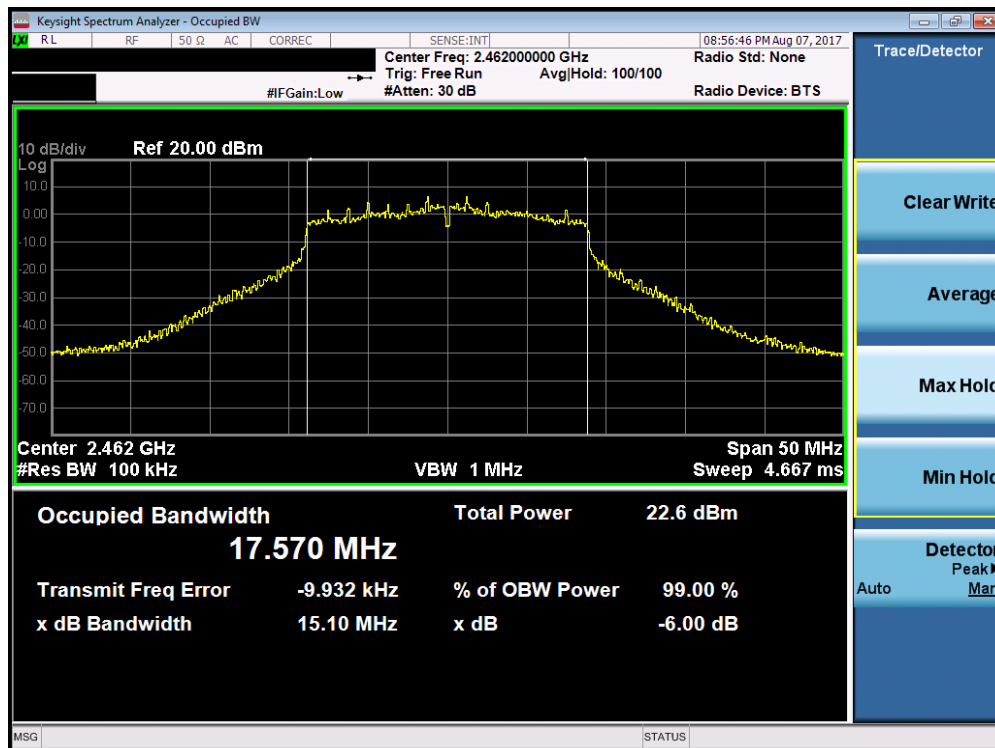
Plot 7-9. 6dB Bandwidth Plot (802.11n (2.4GHz) – Ch. 11)
