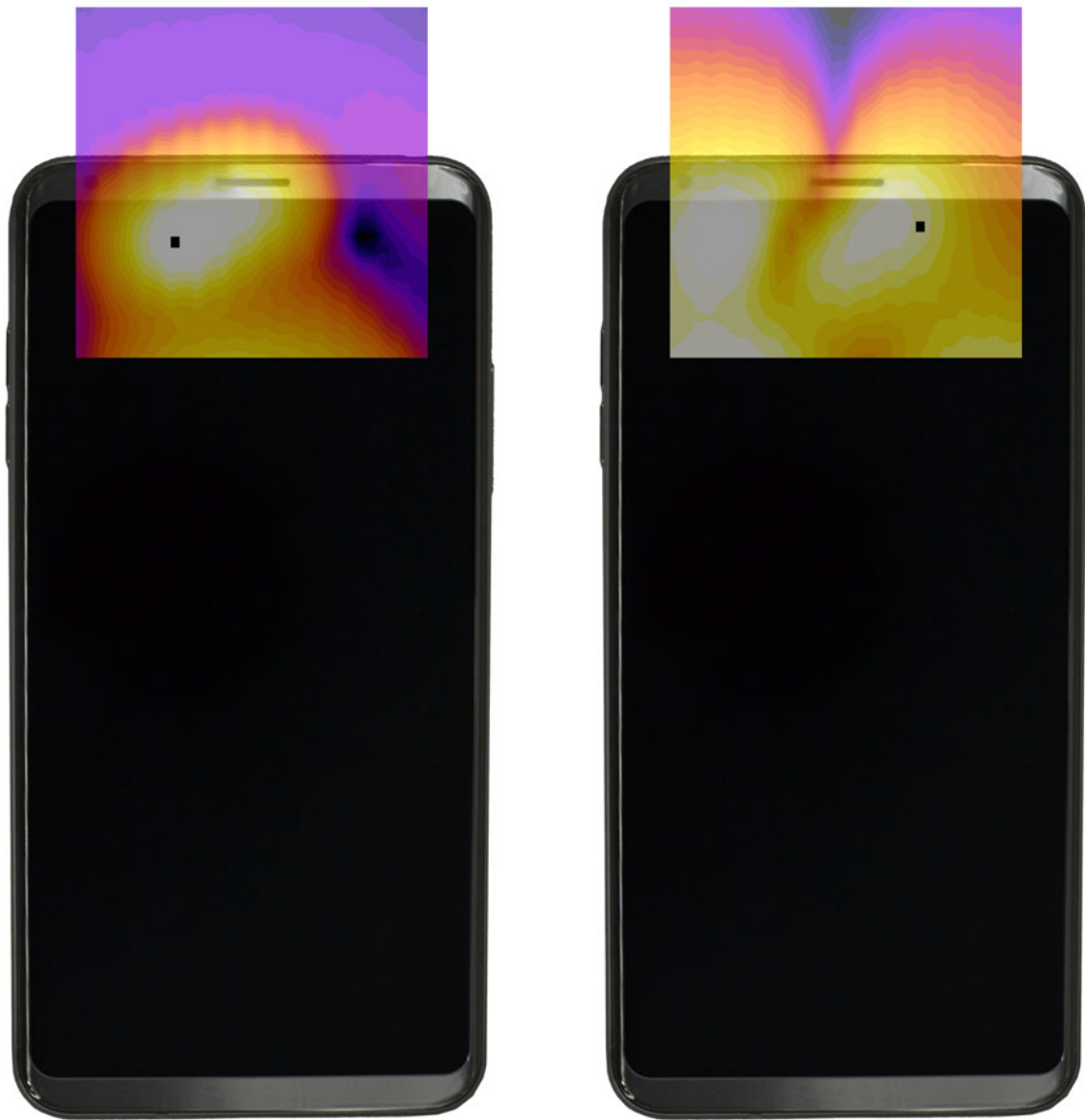
Figure 13-3 T-Coil Scan Overlay Magnetic Field Distributions
