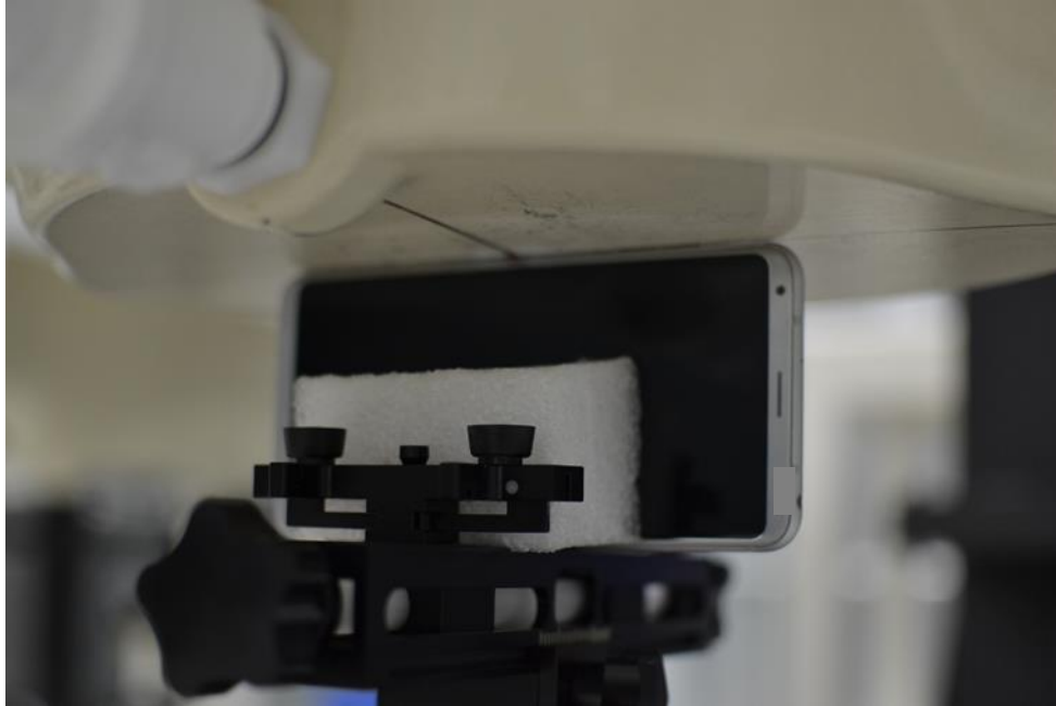
SAR Test Setup Photo 15: Left at 0.0 cm
