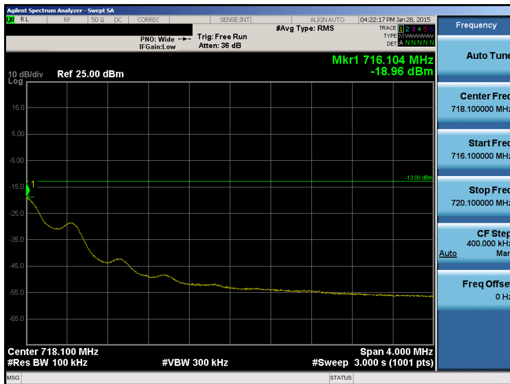
Plot 6-83. Upper Extended Band Edge Plot (Band 12 – 1.4MHz QPSK – RB Size 6)
