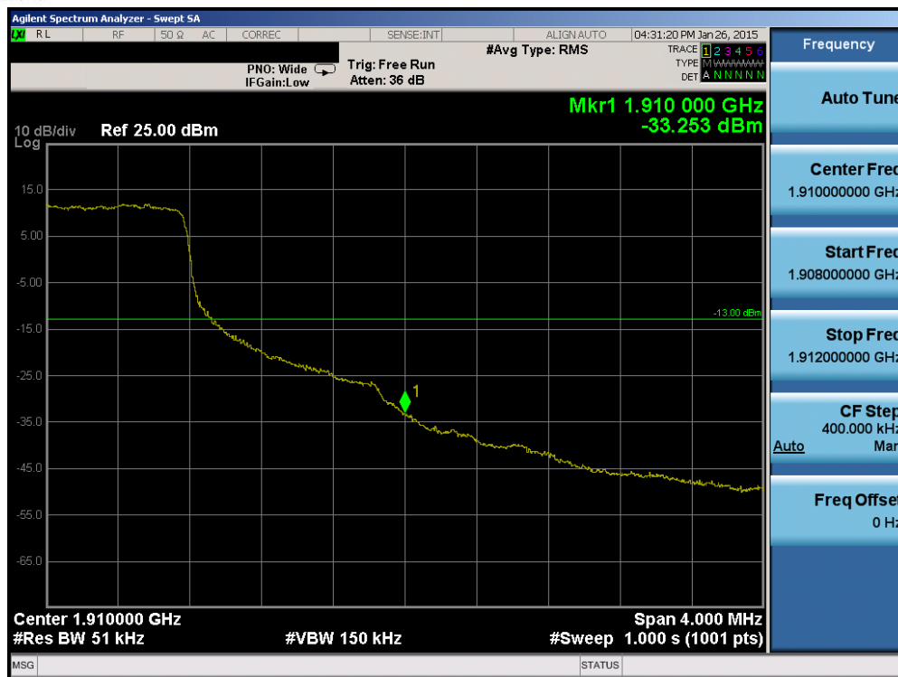
Plot 6-140. Upper Band Edge Plot (Band 2 – 3.0MHz QPSK – RB Size 15)
