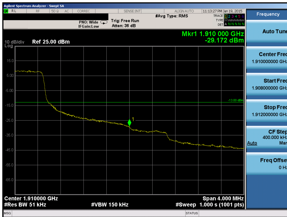
Plot 6-144. Upper Band Edge Plot (Band 2 - 5.0MHz QPSK - RB Size 25)
