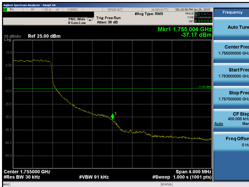
Plot 6-117. Upper Band Edge Plot (Band 4 – 3.0MHz QPSK – RB Size 15)
