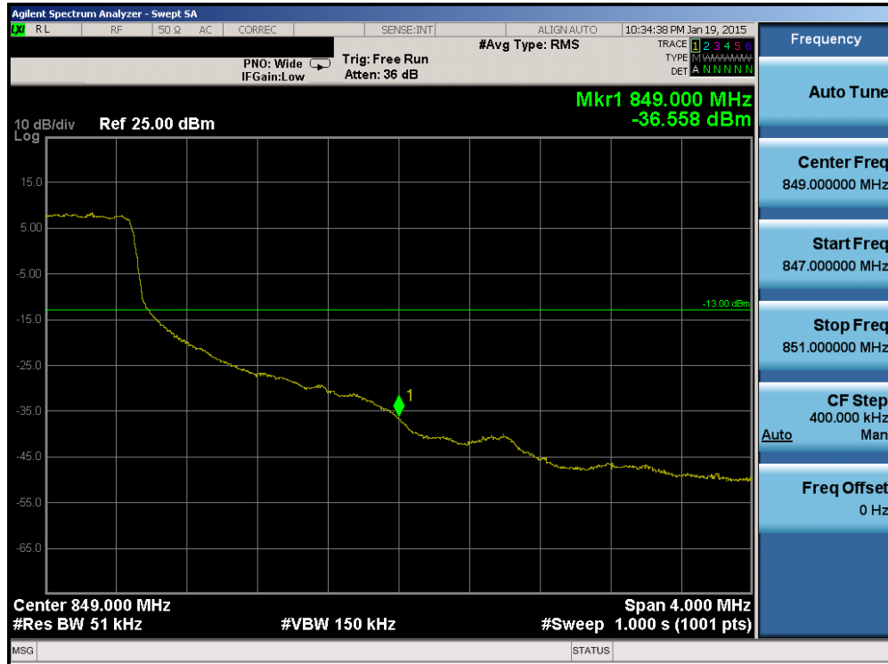
Plot 6-106. Upper Band Edge Plot (Band 5 – 5.0MHz QPSK – RB Size 25)
