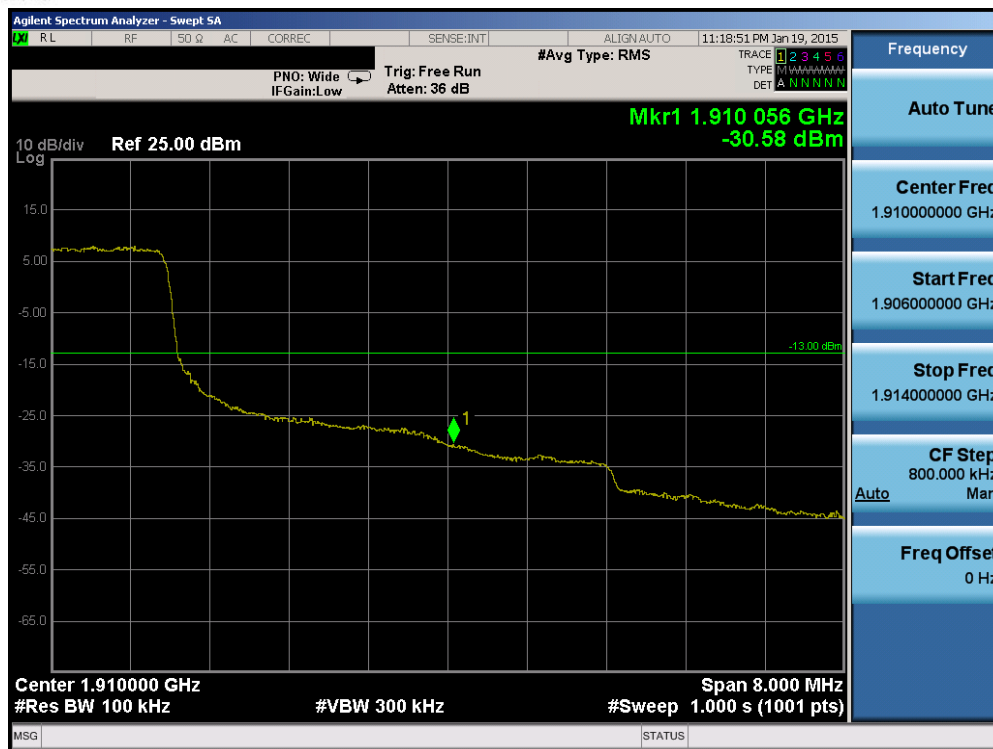
Plot 6-148. Upper Band Edge Plot (Band 2 – 10.0MHz QPSK – RB Size 50)
