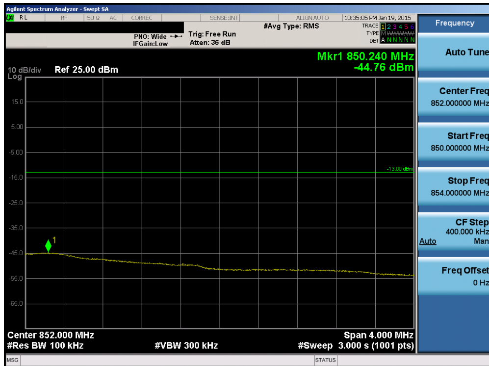
Plot 6-107. Upper Extended Band Edge Plot (Band 5 – 5.0MHz QPSK – RB Size 25)
