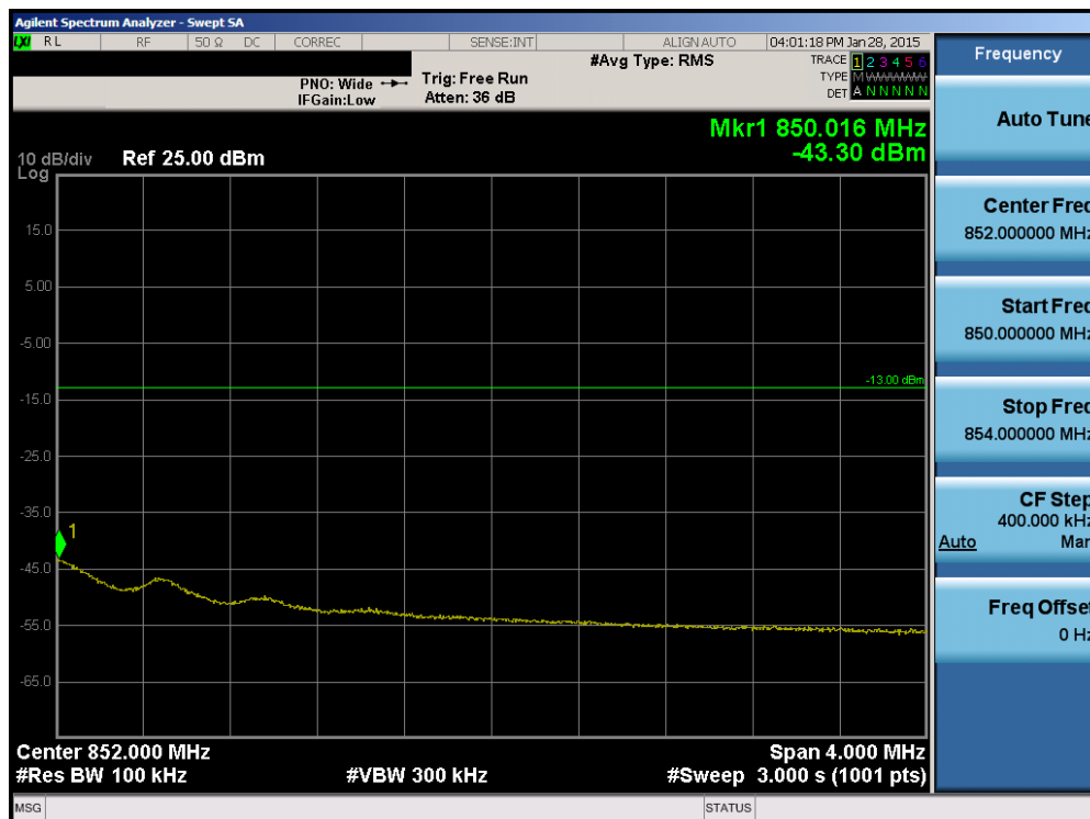
Plot 6-99. Upper Extended Band Edge Plot (Band 5 – 1.4MHz QPSK – RB Size 6)
