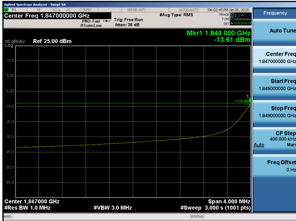
Plot 6-136. Lower Extended Band Edge Plot (Band 2 – 1.4MHz QPSK – RB Size 6)
