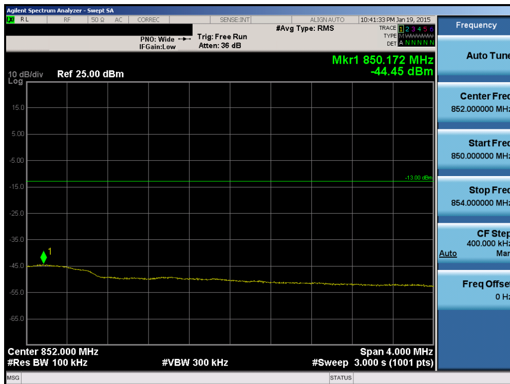
Plot 6-111. Upper Extended Band Edge Plot (Band 5 – 10.0MHz QPSK – RB Size 50)
