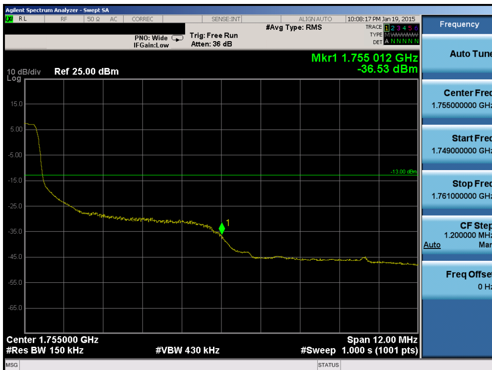
Plot 6-129. Upper Band Edge Plot (Band 4 – 15.0MHz QPSK – RB Size 75)
