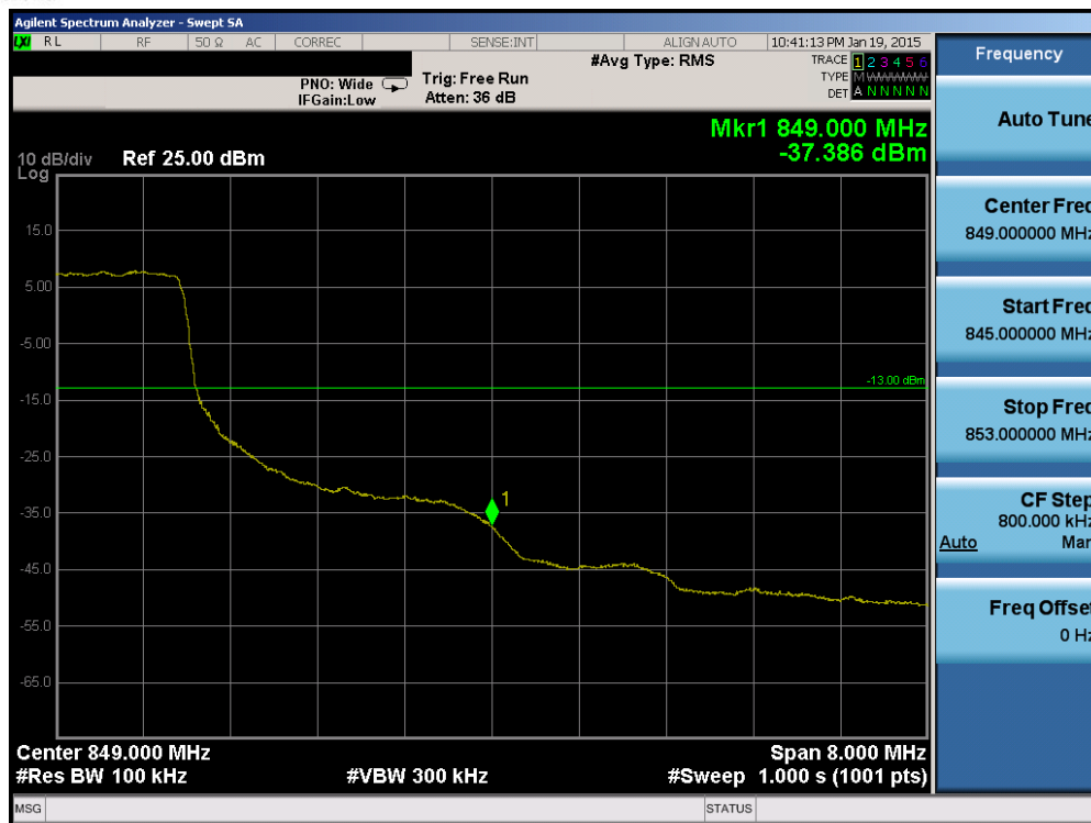
Plot 6-110. Upper Band Edge Plot (Band 5 – 10.0MHz QPSK – RB Size 50)
