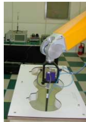
Figure 5. Photograph of the probe and the Phantom
