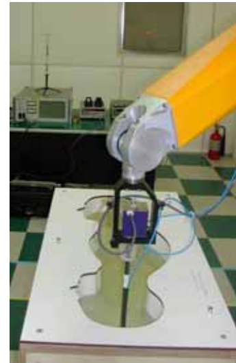
Figure 3. Photograph of the probe and the Phantom
