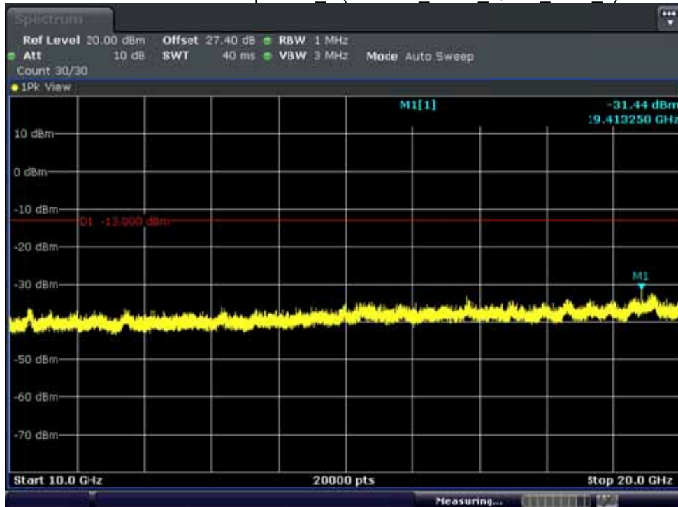
BAND 2. Conducted Spurious_2 (19175ch_5MHz_QPSK_RB 1_0)
