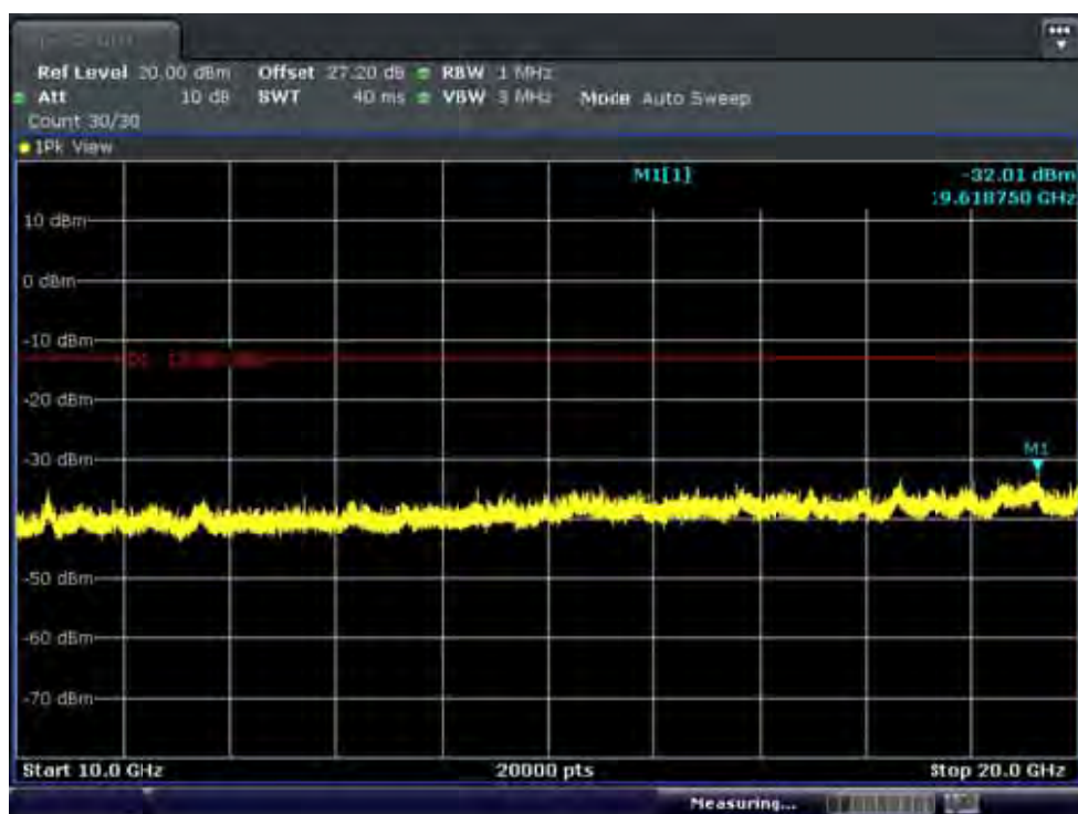
BAND 4. Conducted Spurious Plot_2 (20175ch_3MHz_QPSK_RB 1_0)
