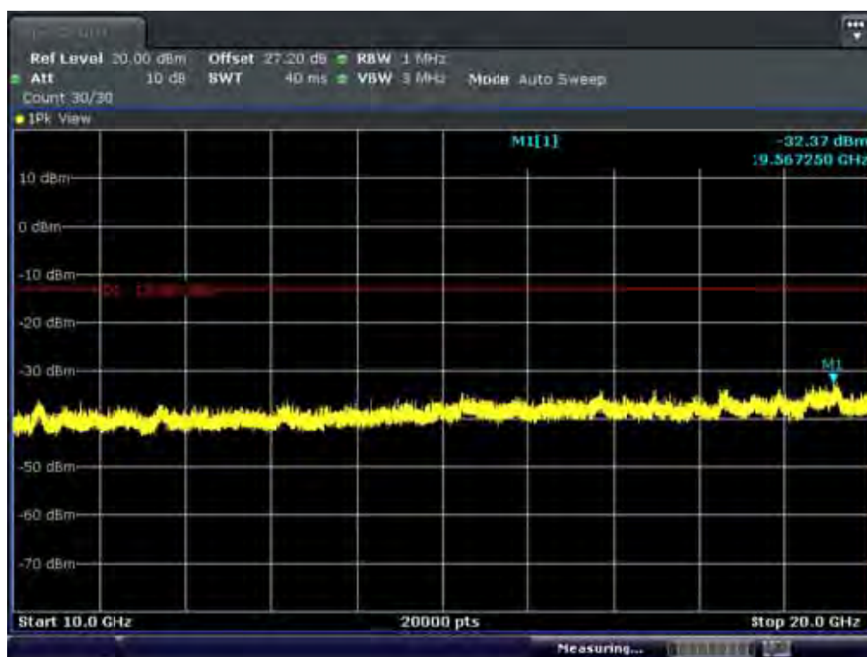
BAND 4. Conducted Spurious Plot_2 (19975ch_5MHz_QPSK_RB 1_0)
