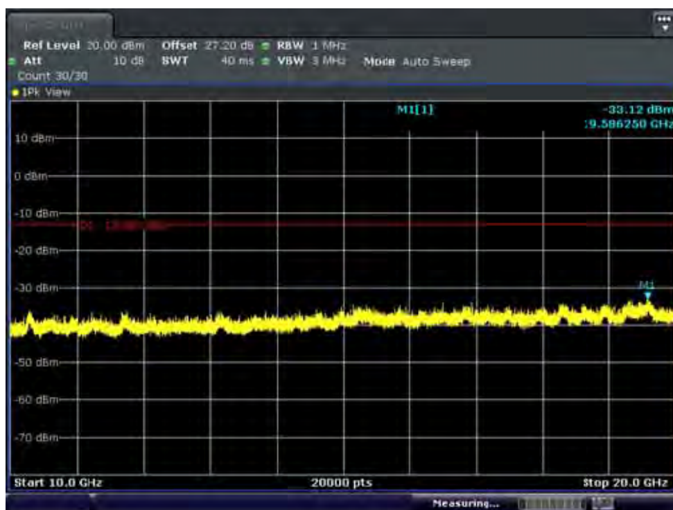
BAND 4. Conducted Spurious Plot_2 (20175ch_20MHz_QPSK_ RB 1_0)
