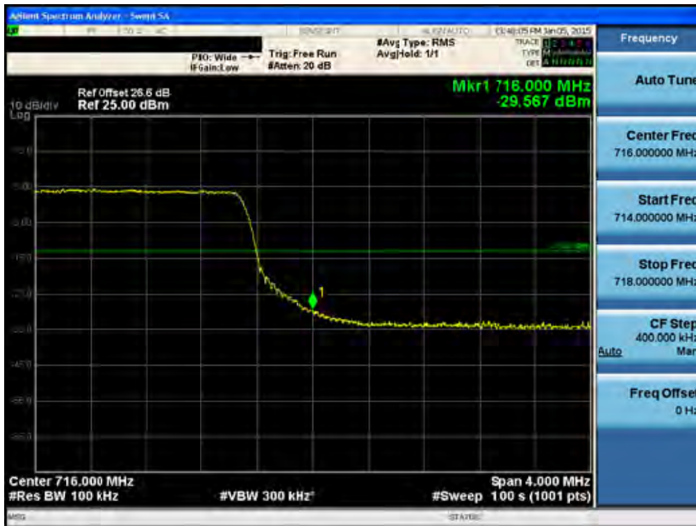
Band 17 Upper Band Edge Plot (10M BW Ch.23800 QPSK_RB50)
