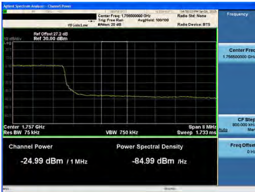
BAND 4. Upper Extended Band Edge Plot (10M BW Ch.20350 QPSK_RB50) -3
