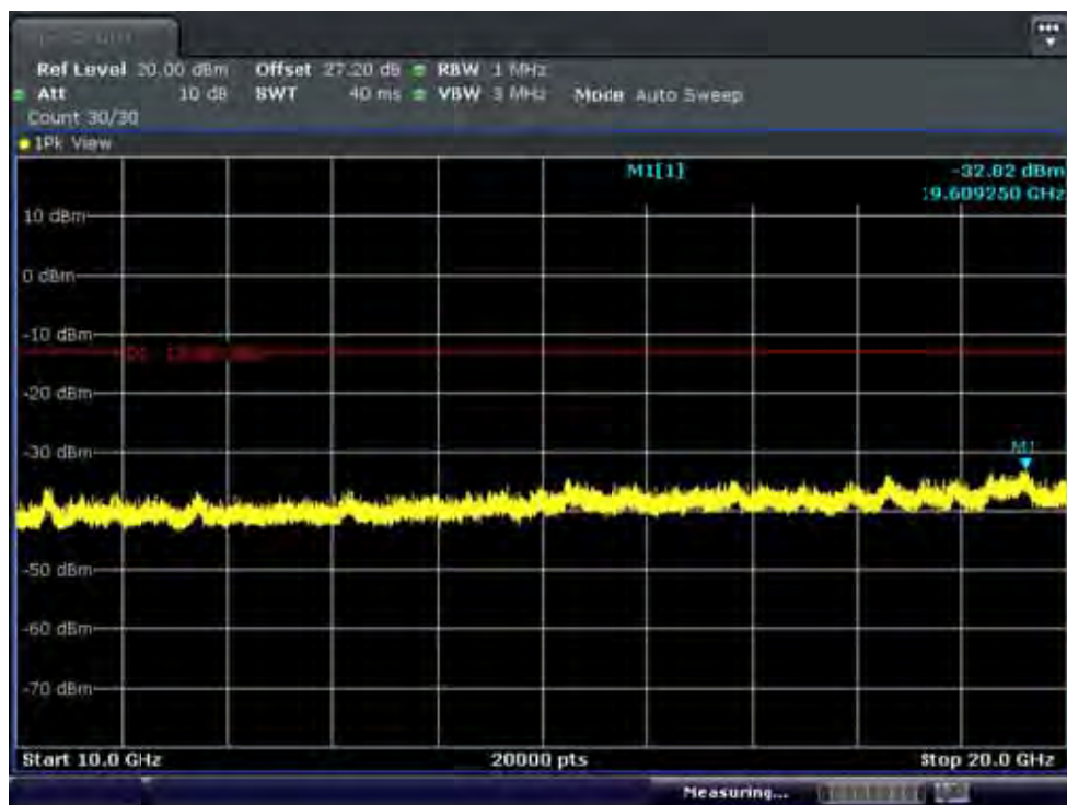
BAND 4 . Conducted Spurious Plot_2 (20393ch_1.4MHz_QPSK_ RB 1_0)
