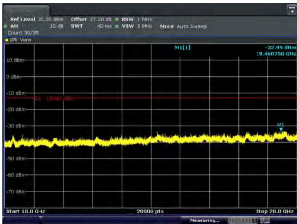
BAND 4. Conducted Spurious Plot_2 (20025ch_15MHz_QPSK_ RB 1_0)
