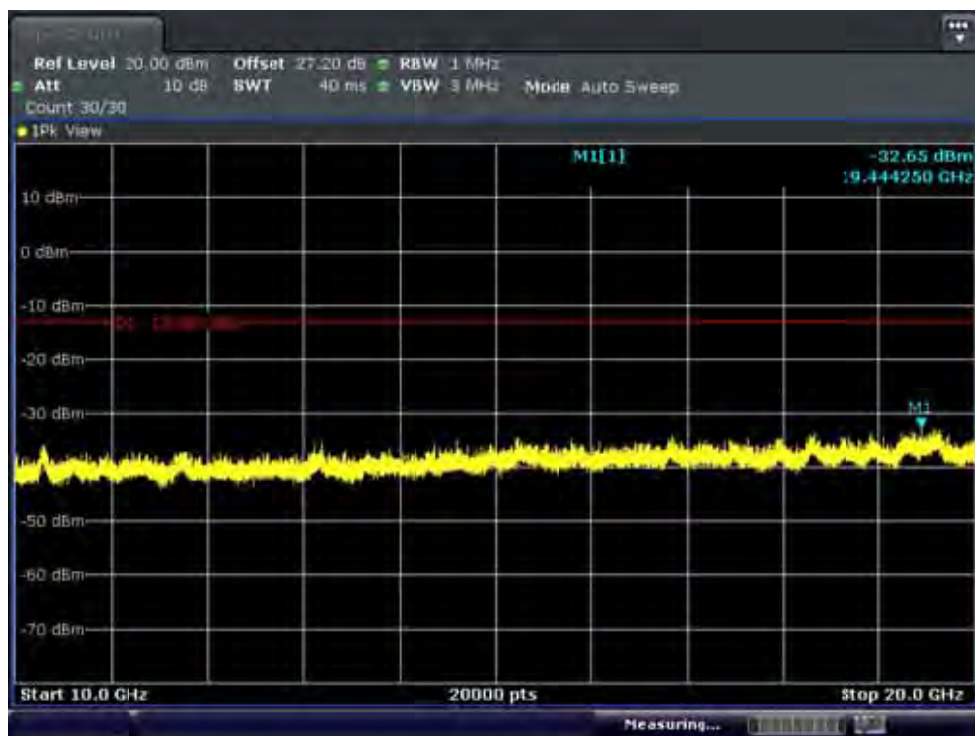
BAND 4 . Conducted Spurious Plot_2 (20325ch_15MHz_QPSK_ RB 1_0)
