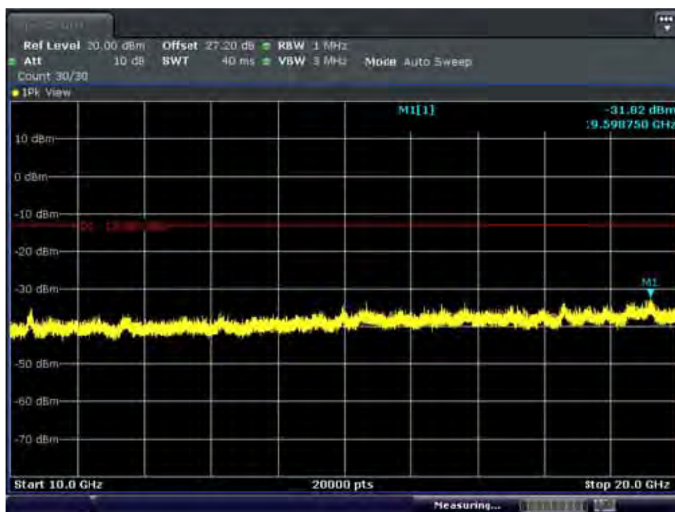
BAND 4. Conducted Spurious Plot_2 (19965ch_3MHz_QPSK_RB 1_0)
