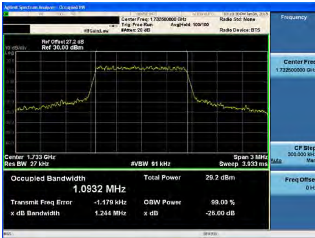
BAND 4. Occupied Bandwidth Plot (1.4M BW Ch.20175 QPSK RB 6)
