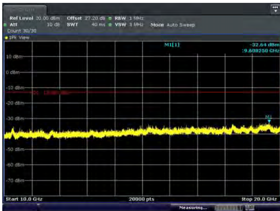
BAND 4. Conducted Spurious Plot_2 (20175ch_15MHz_QPSK_ RB 1_0)
