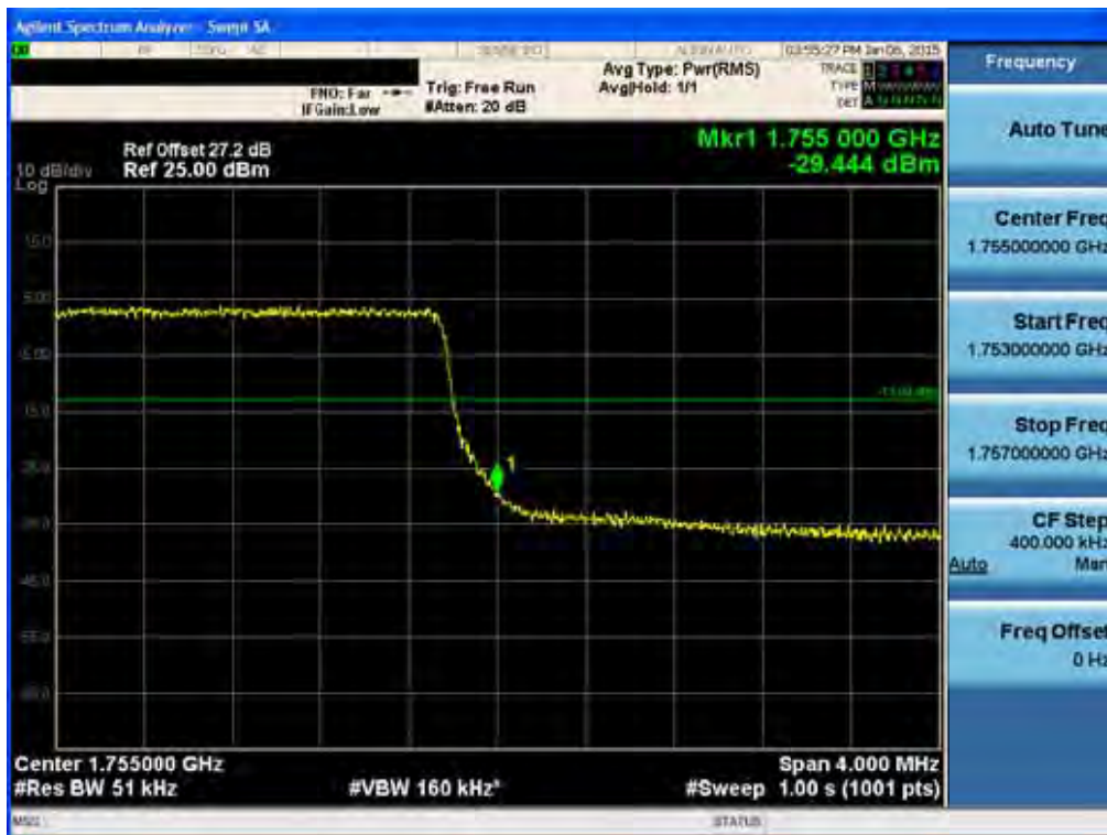
BAND 4. Upper Band Edge Plot (5M BW Ch.20375 QPSK_RB25) -2
