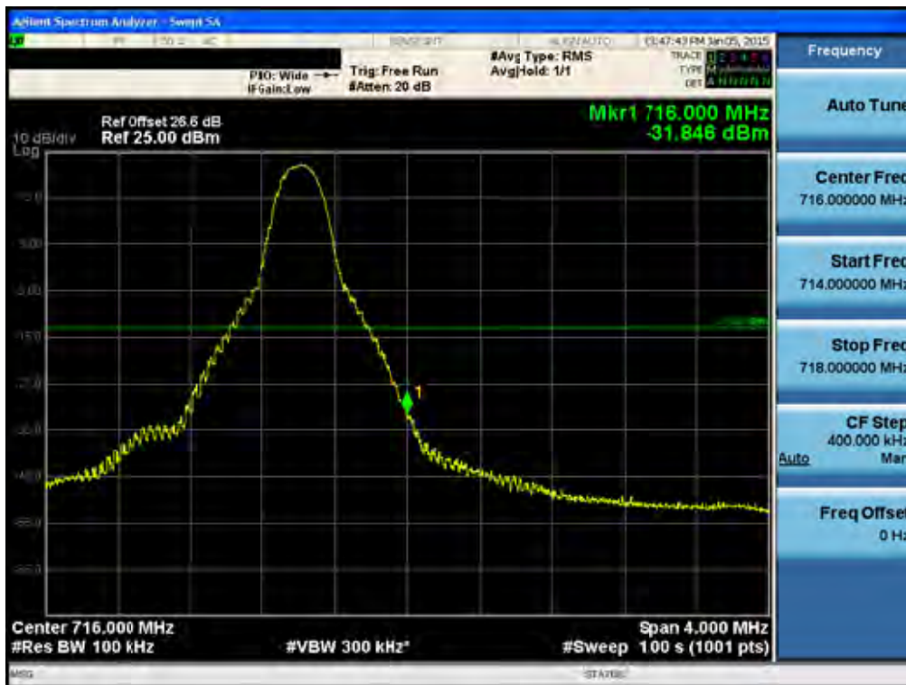
Band 17 Upper Band Edge Plot (10M BW Ch.23800 QPSK_RB1_Offset 49)
