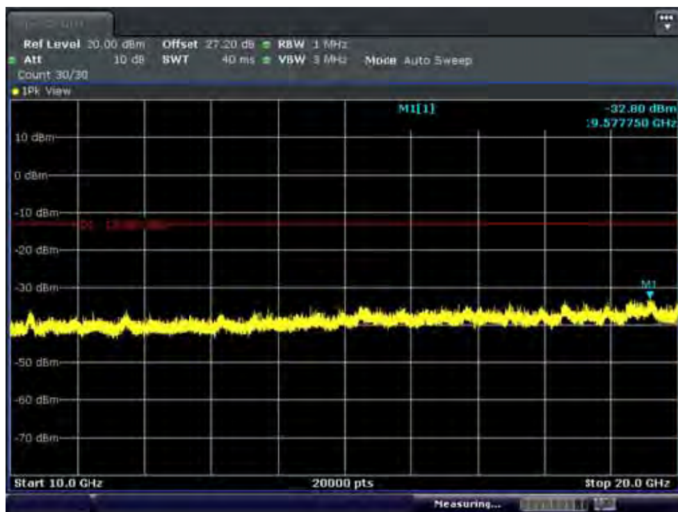
BAND 4. Conducted Spurious Plot_2 (20000ch_10MHz_QPSK_ RB 1_0)
