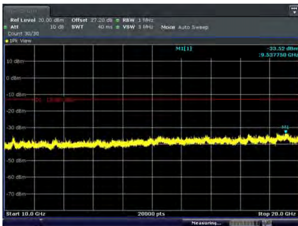
BAND 4. Conducted Spurious Plot_2 (19957ch_1.4MHz_QPSK_RB 1_0)
