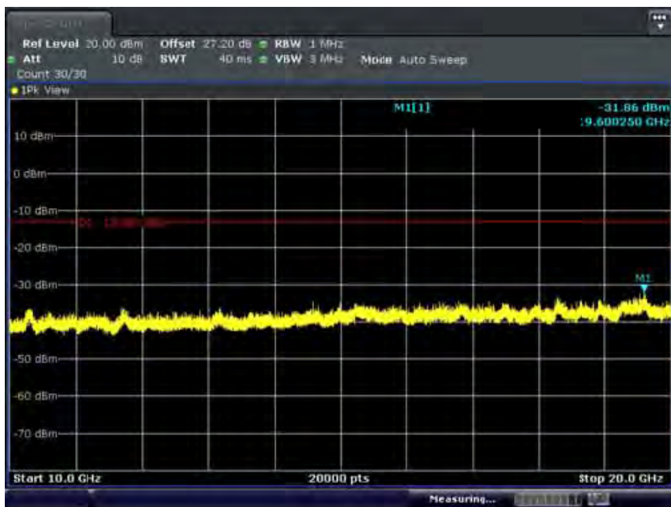
BAND 4. Conducted Spurious Plot_2 (20175ch_5MHz_QPSK_RB 1_0)
