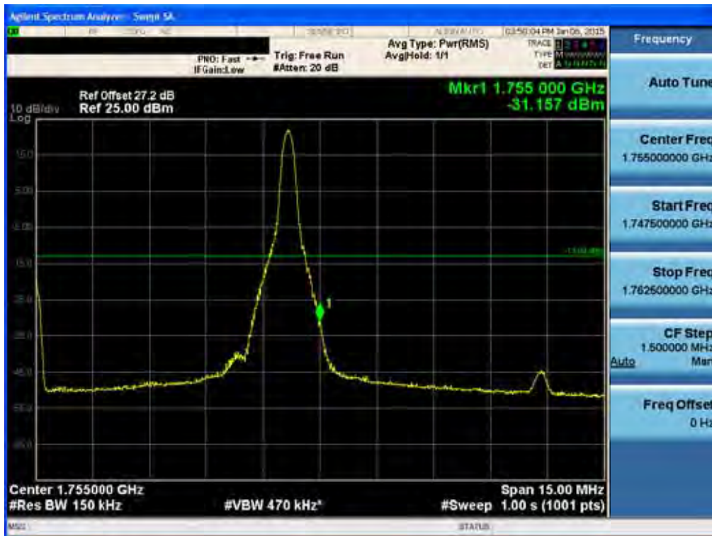
BAND 4. Upper Band Edge Plot (15M BW Ch.20325 QPSK_RB1_Offset 74) -1
