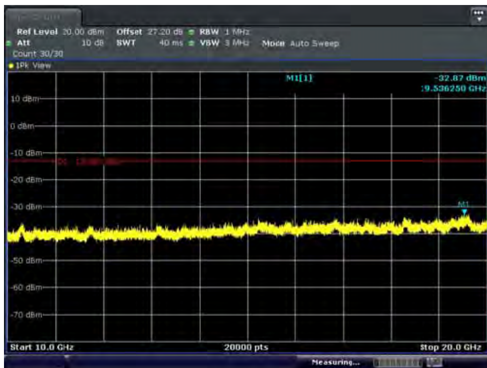
BAND 4. Conducted Spurious Plot_2 (20350ch_10MHz_QPSK_ RB 1_0)
