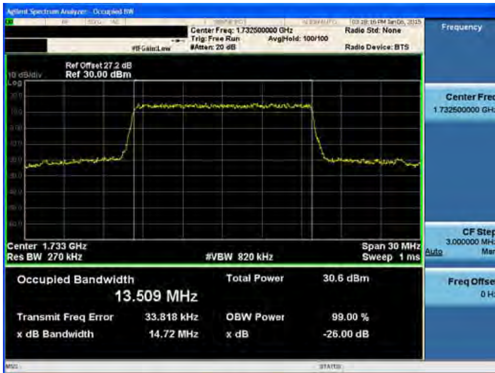
BAND 4. Occupied Bandwidth Plot (15M BW Ch.20175 QPSK RB 75)
