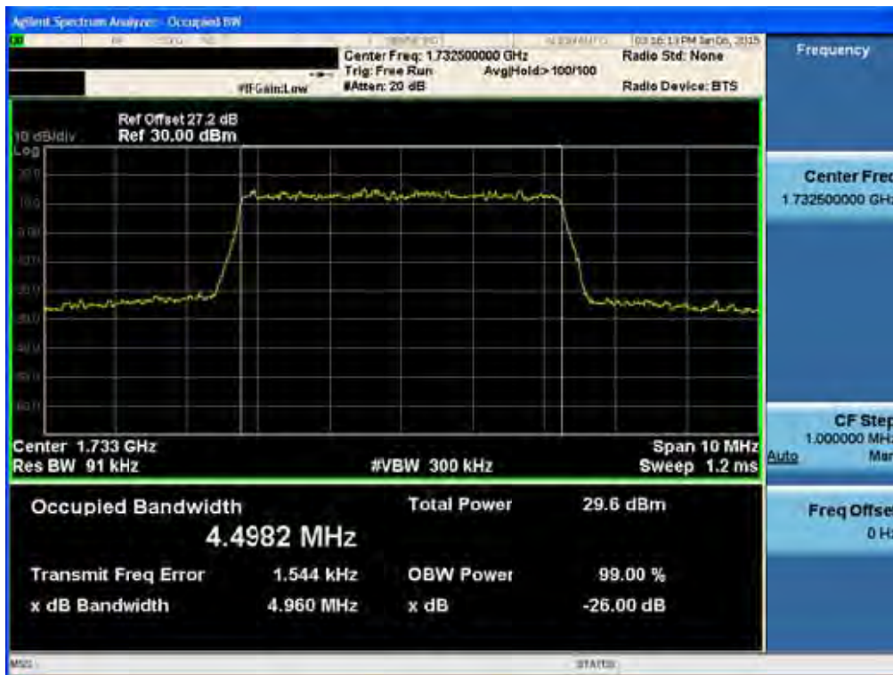
BAND 4. Occupied Bandwidth Plot (5M BW Ch.20175 16QAM RB 25)
