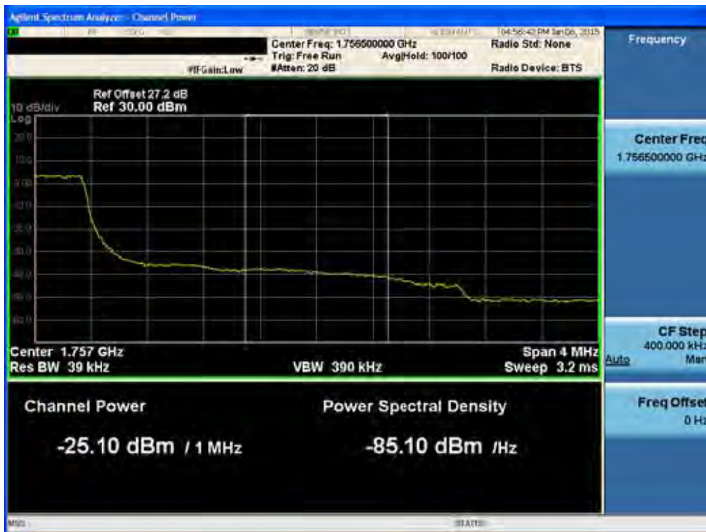
BAND 4. Upper Extended Band Edge Plot (3M BW Ch.20385 QPSK_RB15_0) -3
