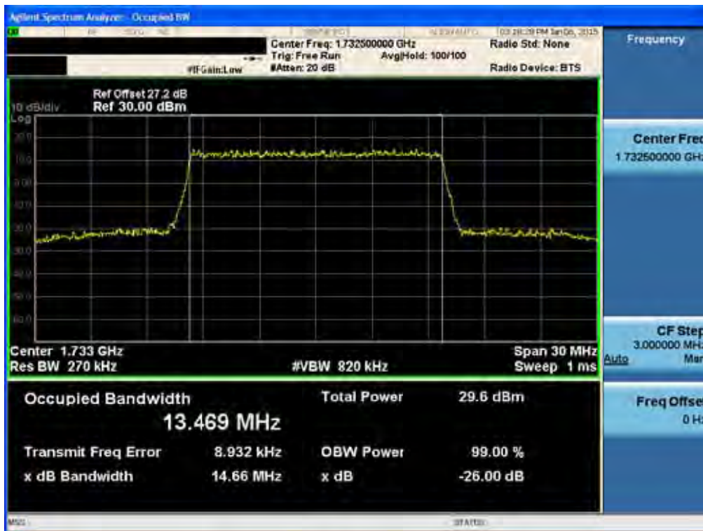
BAND 4. Occupied Bandwidth Plot (15M BW Ch.20175 16QAM RB 75)
