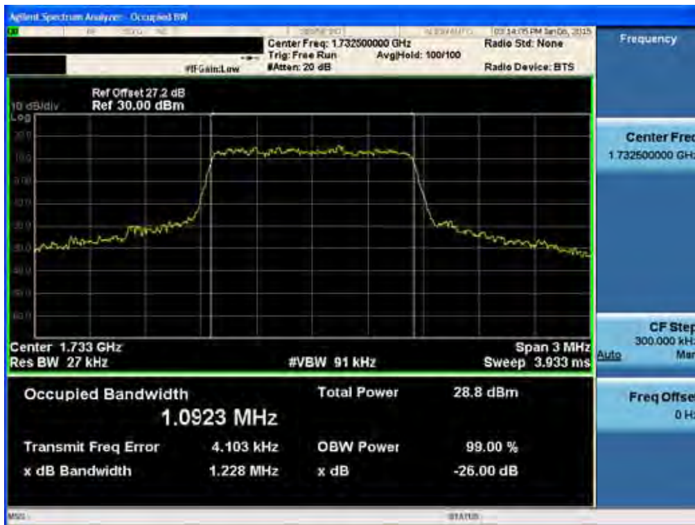
BAND 4. Occupied Bandwidth Plot (1.4M BW Ch.20175 16QAM RB 6)
