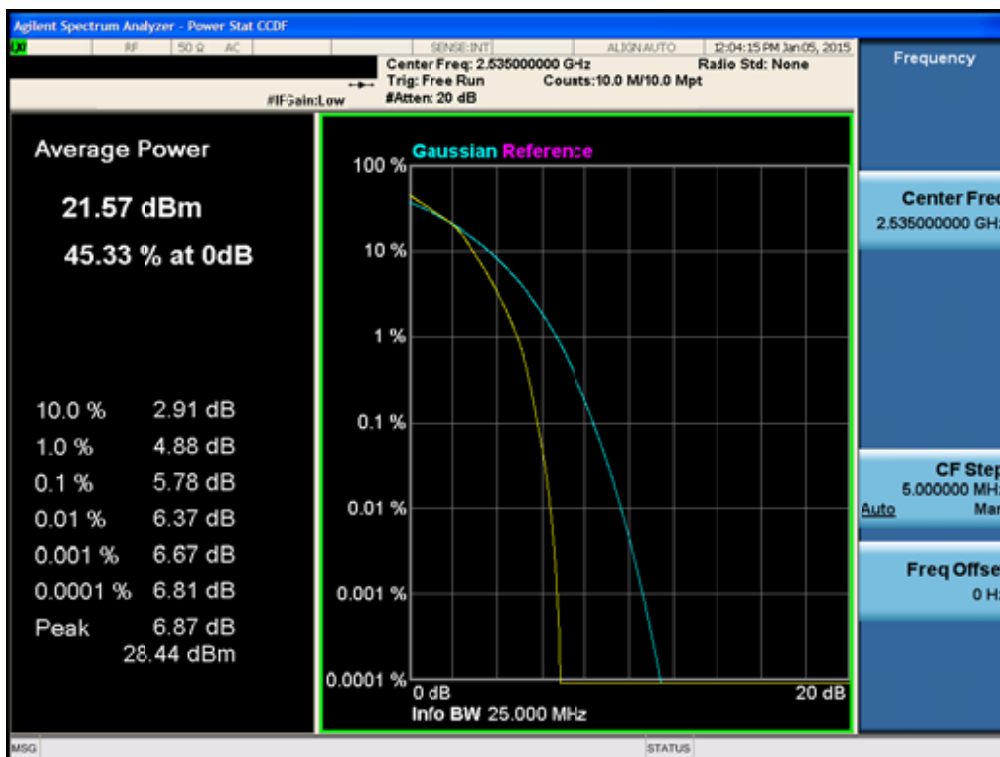
BAND7. Peak to Average Ratio Plot (20MHz Ch.21100 16-QAM RB 100)
