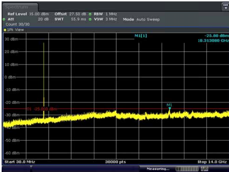
BAND7. Conducted Spurious Plot 1 (20MHz Ch.21100 QPSK RB 1, Offset 0)
