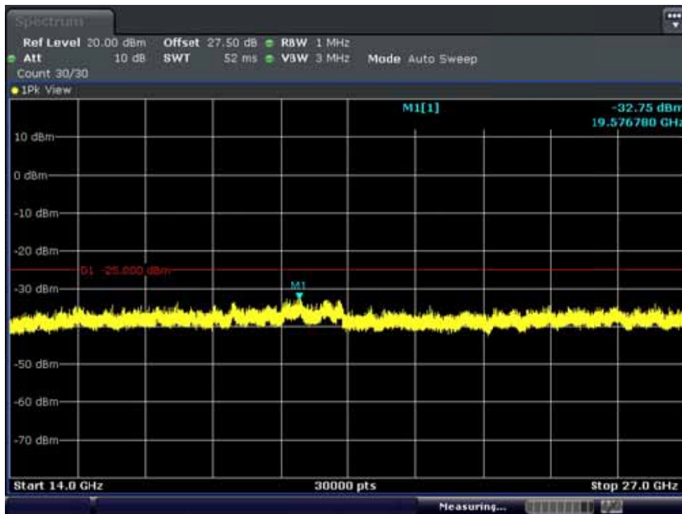
BAND7. Conducted Spurious Plot 2 (5MHz Ch.20775 QPSK RB 1, Offset 0)
