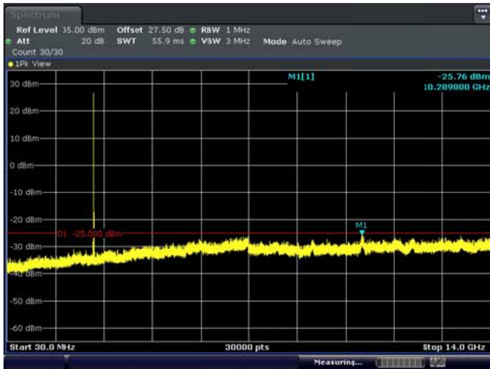
BAND7. Conducted Spurious Plot 1 (15MHz Ch.21100 QPSK RB 1, Offset 0)
