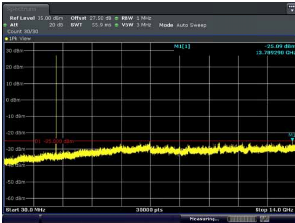
BAND7. Conducted Spurious Plot 1 (5MHz Ch.20775 QPSK RB 1, Offset 0)
