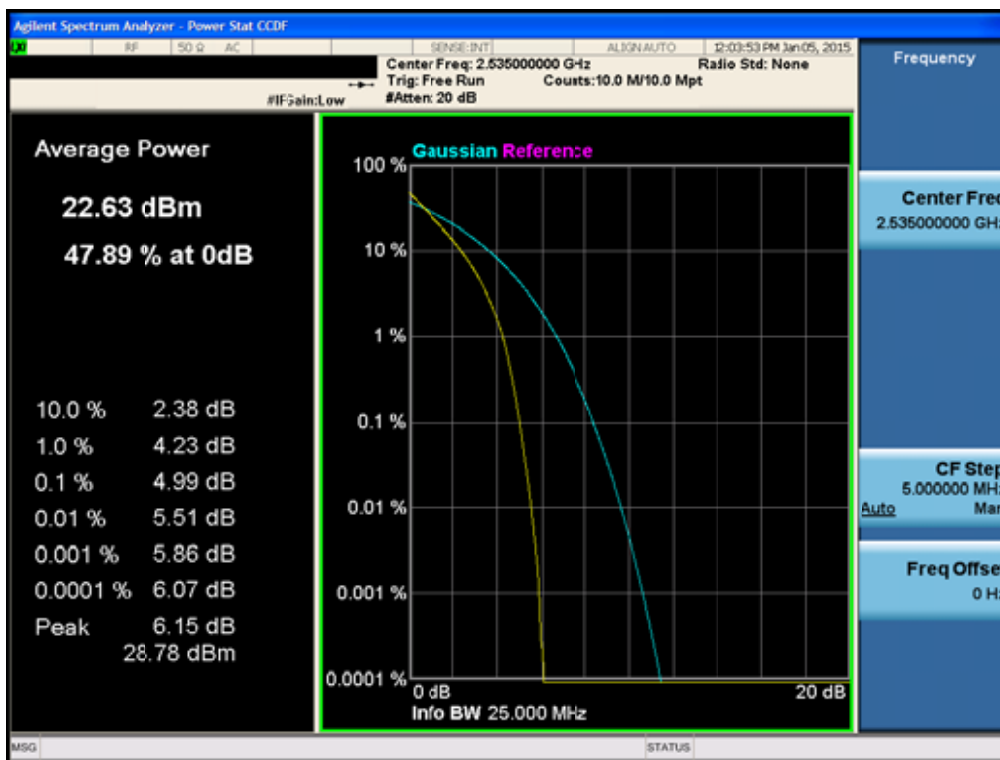
BAND7. Peak to Average Ratio Plot (20MHz Ch.21100 QPSK RB 100)
