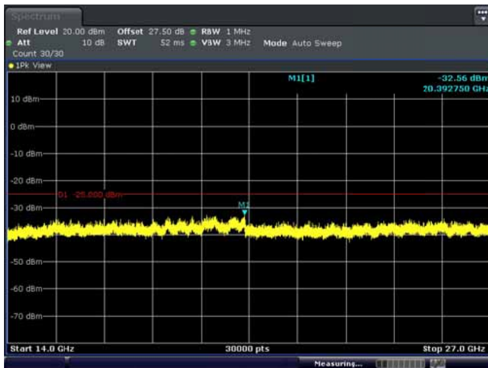
BAND7. Conducted Spurious Plot 2 (20MHz Ch.21350 QPSK RB 1, Offset 0)
