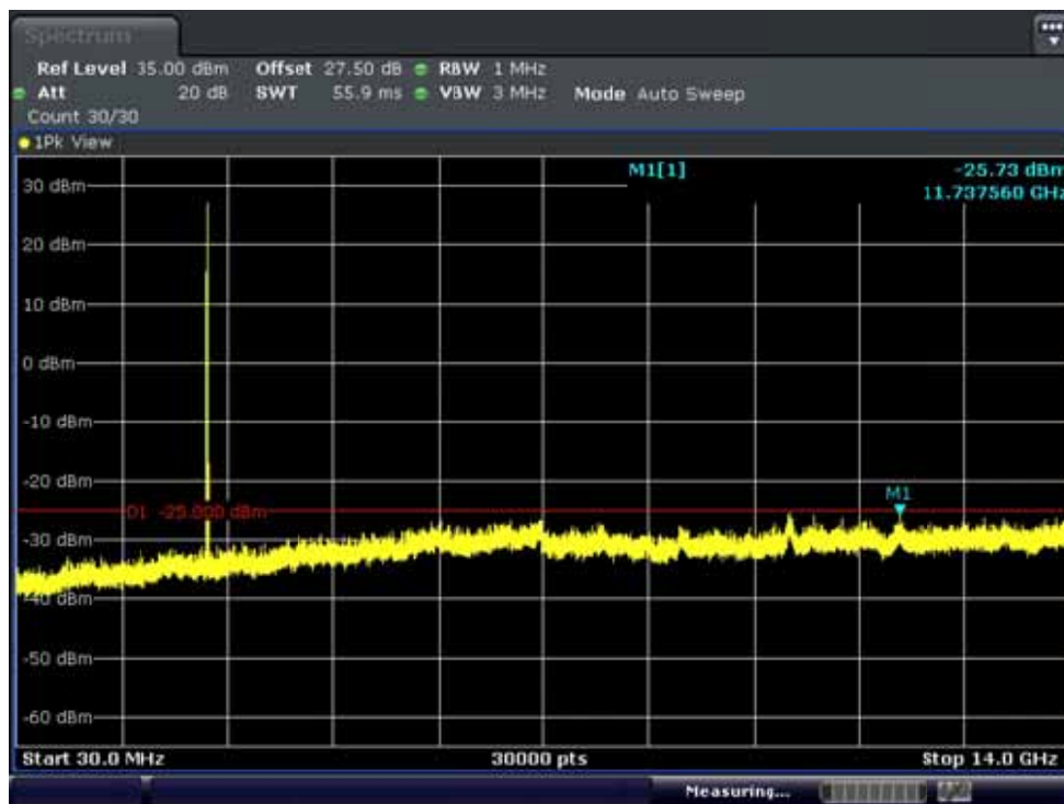
BAND7. Conducted Spurious Plot 1 (20MHz Ch.21350 QPSK RB 1, Offset 0)
