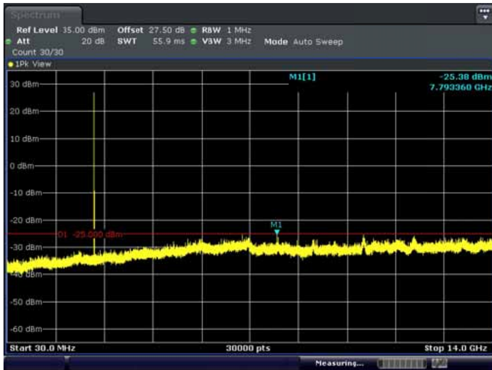
BAND7. Conducted Spurious Plot 1 (10MHz Ch.21100 QPSK RB 1, Offset 0)
