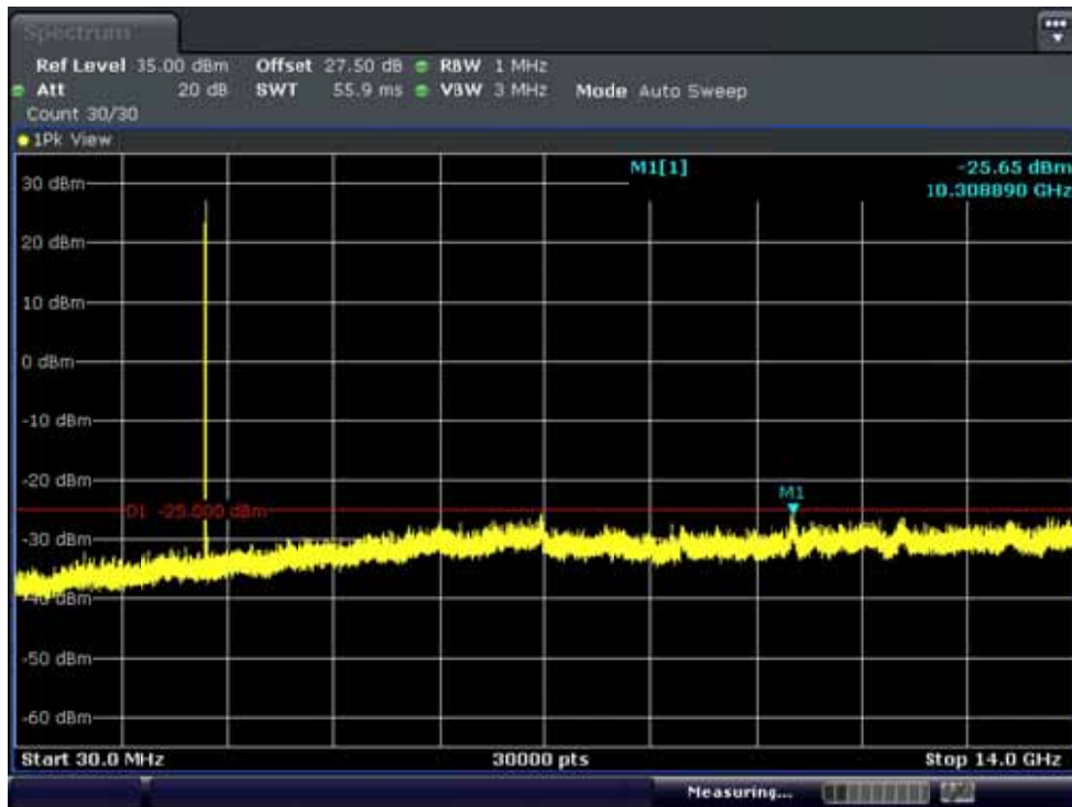
BAND7. Conducted Spurious Plot 1 (5MHz Ch.21100 QPSK RB 1, Offset 0)
