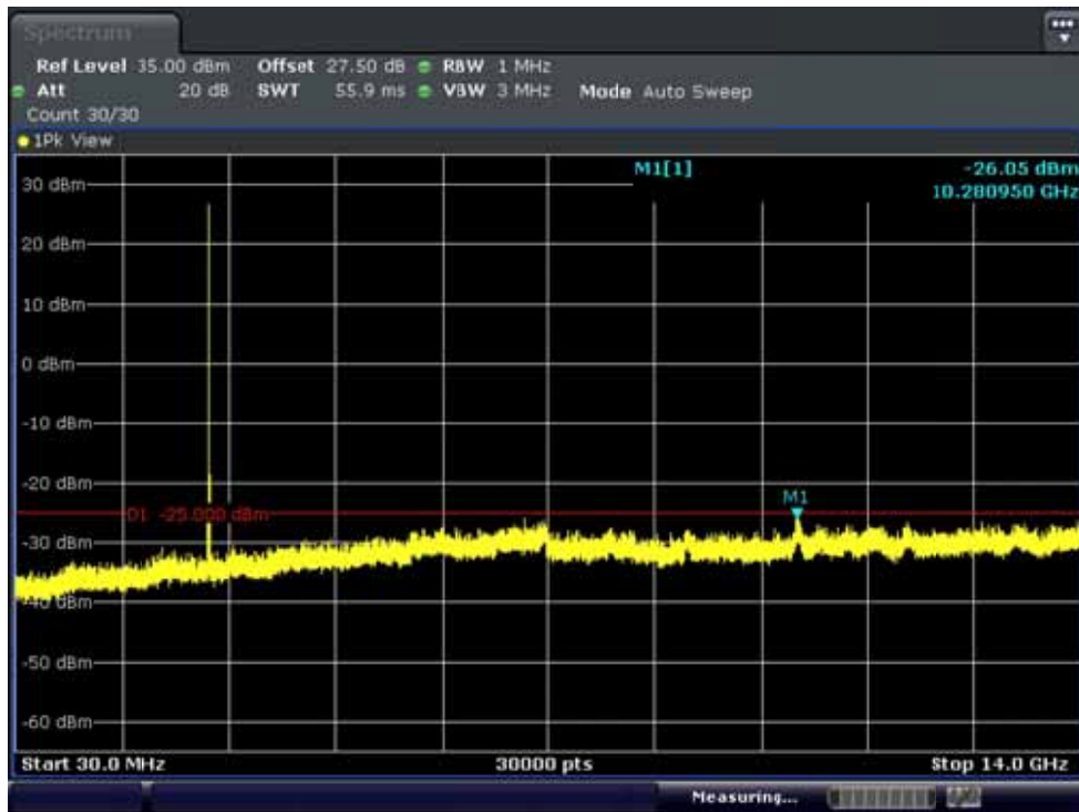
BAND7. Conducted Spurious Plot 1 (15MHz Ch.21375 QPSK RB 1, Offset 0)
