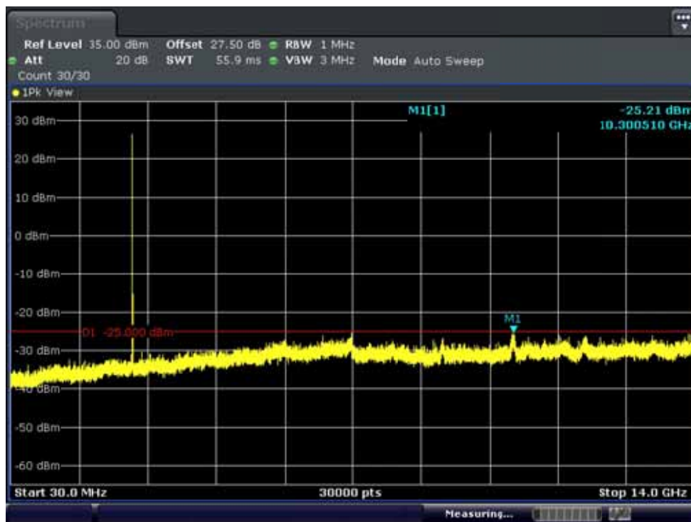
BAND7. Conducted Spurious Plot 1 (20MHz Ch.20850 QPSK RB 1, Offset 0)
