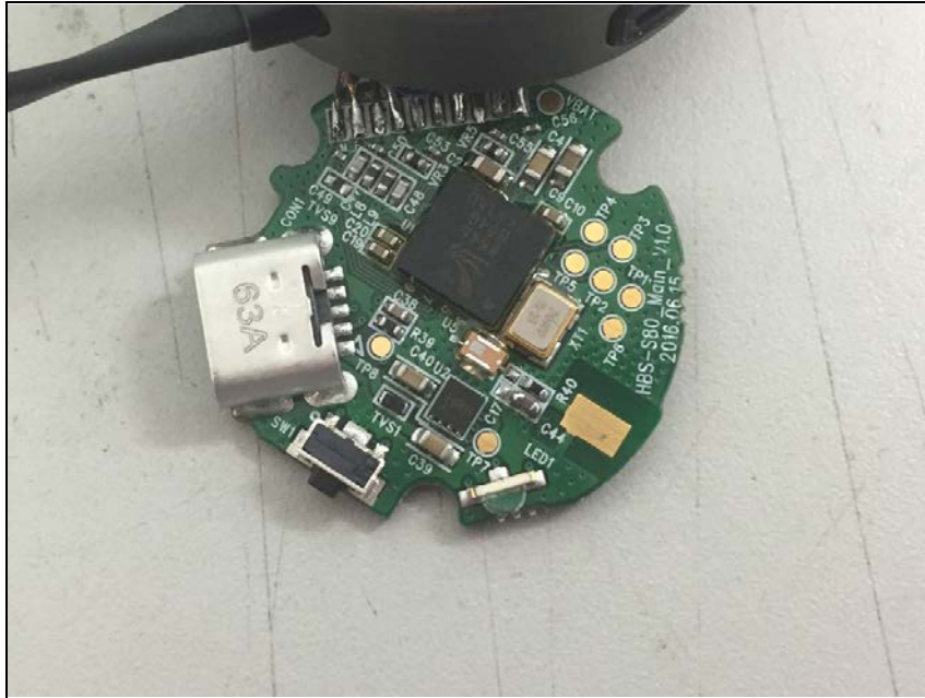
Top view of Main PCB (Left earbud)
