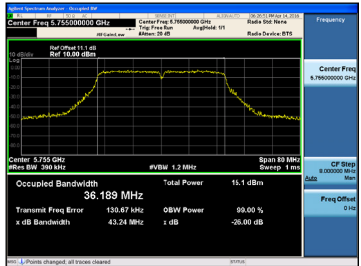
802.11n_HT40UNII 3 BAND 26dB Bandwidth (CH 151)
