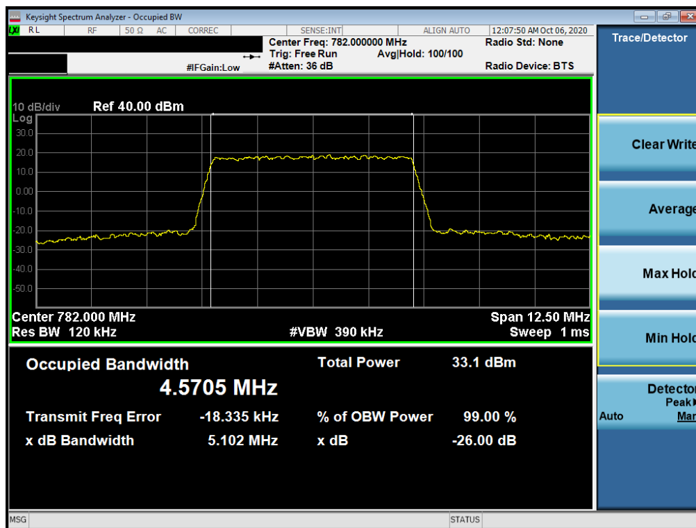
Plot 7-16. Occupied Bandwidth Plot (LTE Band 13 - 5MHz QPSK - Full RB Configuration)
