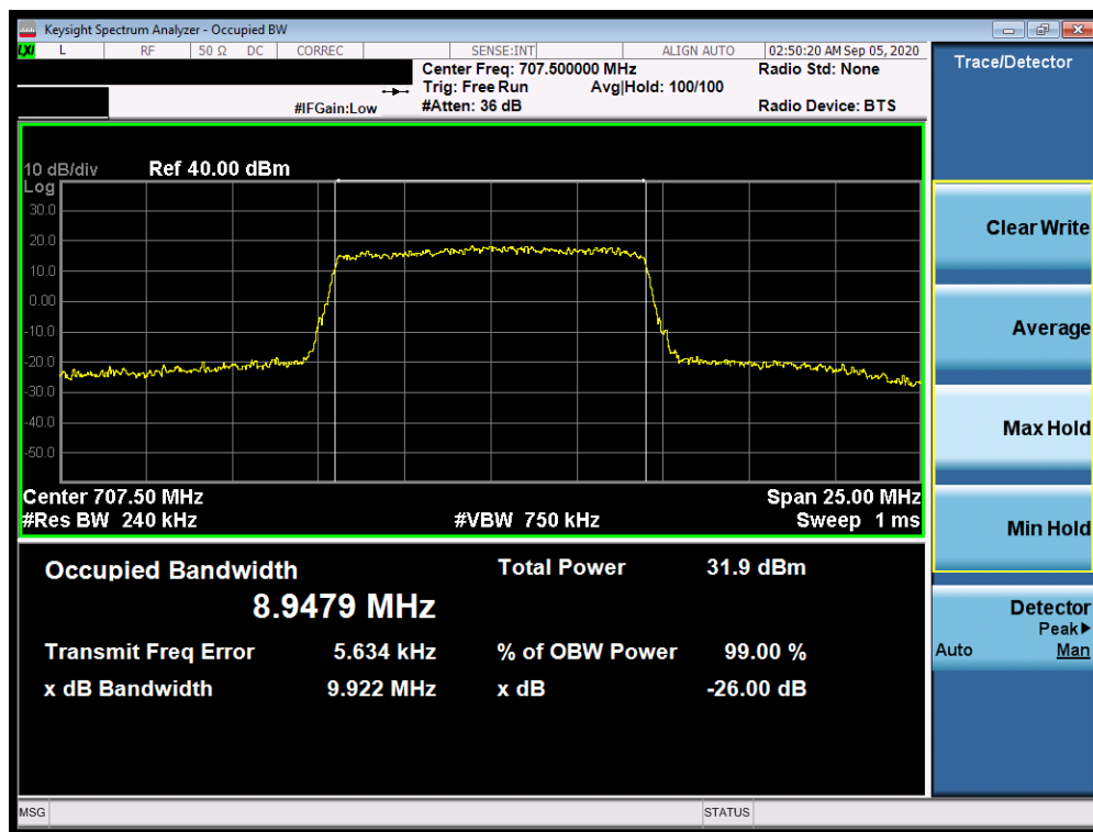
Plot 7-1. Occupied Bandwidth Plot (LTE Band 12/17 - 10MHz QPSK - Full RB Configuration)
