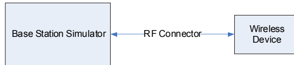
Figure 9-2 Power Measurement Setup
