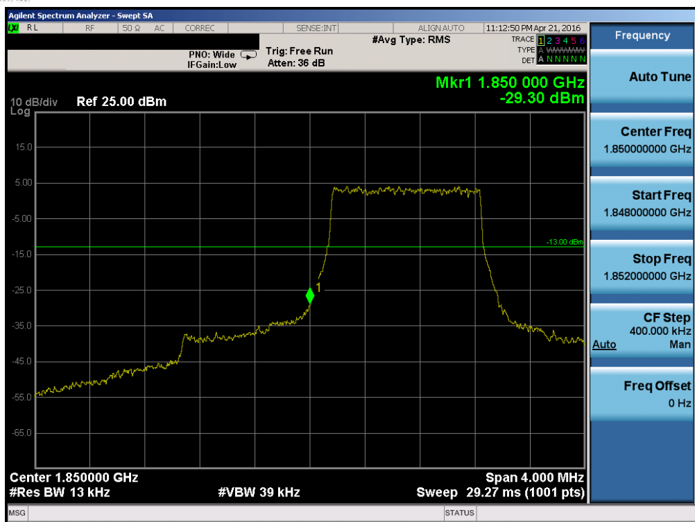
Plot 7-129. Lower Band Edge Plot (Band 2 – 1.4MHz QPSK – RB Size 6)
