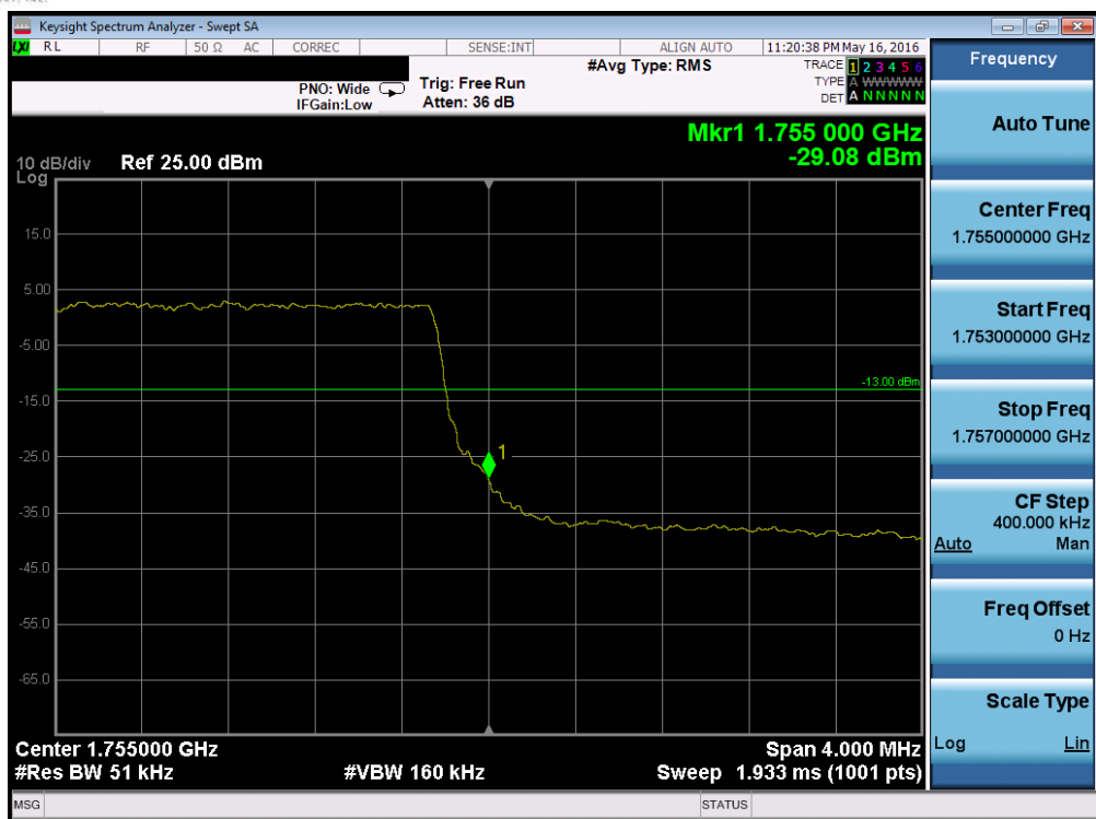
Plot 7-115. Upper Band Edge Plot (Band 4 – 5.0MHz QPSK – RB Size 25)
