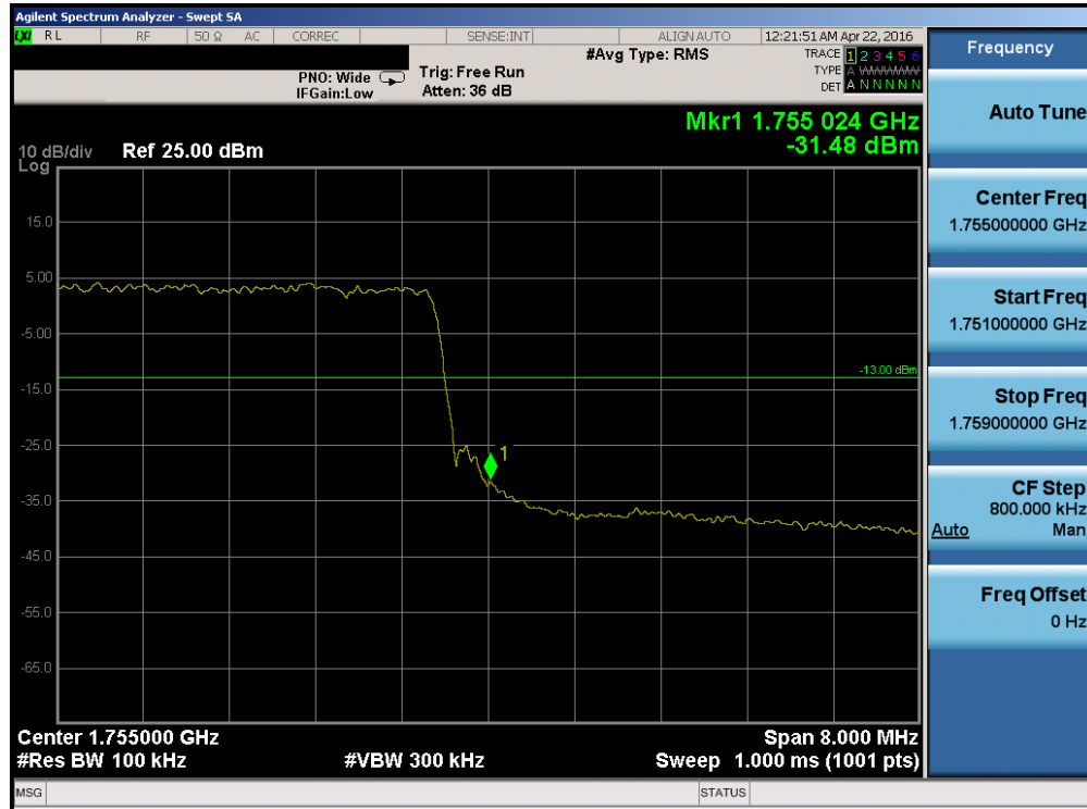
Plot 7-119. Upper Band Edge Plot (Band 4 – 10.0MHz QPSK – RB Size 50)
