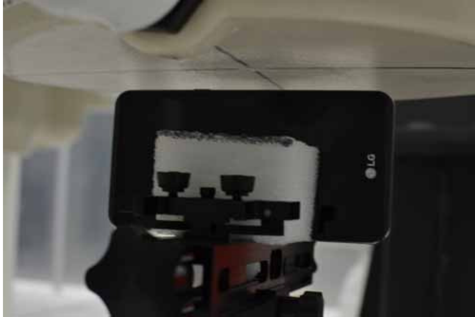
SAR Test Setup Photo 9 - Right at 10mm
