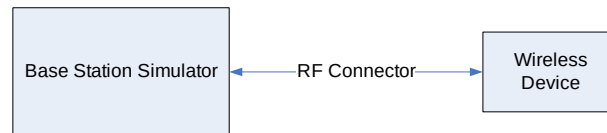
Figure 9-3 Power Measurement Setup
