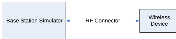
Figure 9-1 Power Measurement Setup
