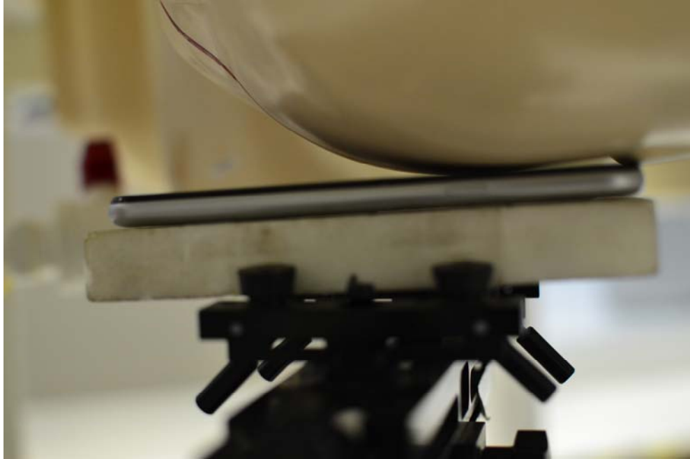
SAR Test Setup Photo 1: Left Cheek
