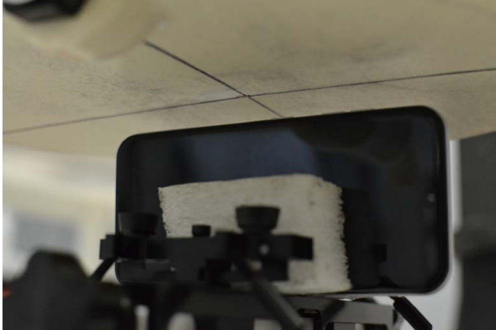
SAR Test Setup Photo 9: Left Edge at 10 mm
