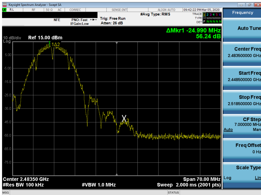
Plot 7-20. Band Edge Plot (802.11b – Ch. 11)
