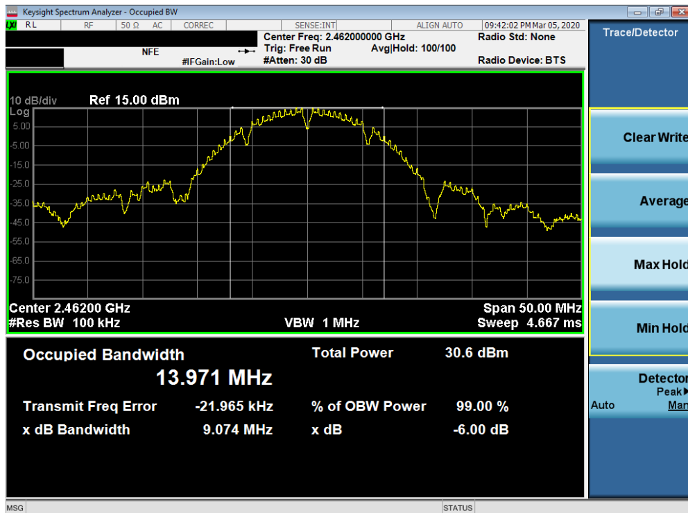
Plot 7-3. 6dB Bandwidth Plot (802.11b – Ch. 11)
