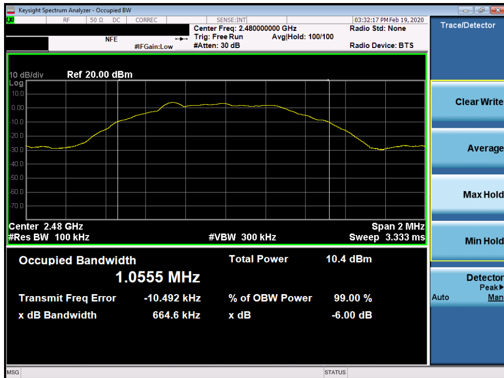
Plot 7-6. 6dB Bandwidth Plot (Bluetooth (LE), 500kbps – Ch. 39)
